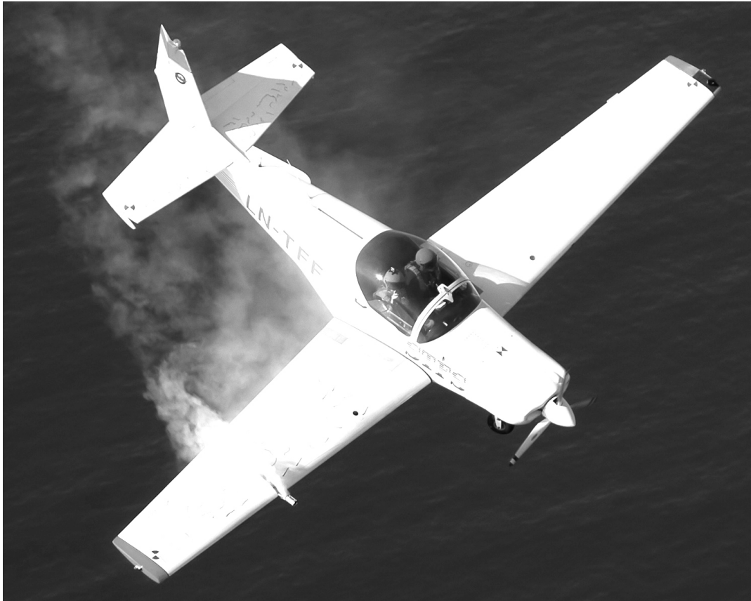
Figure 59. Smoke visualization before the 1-turn point in the left spin.
