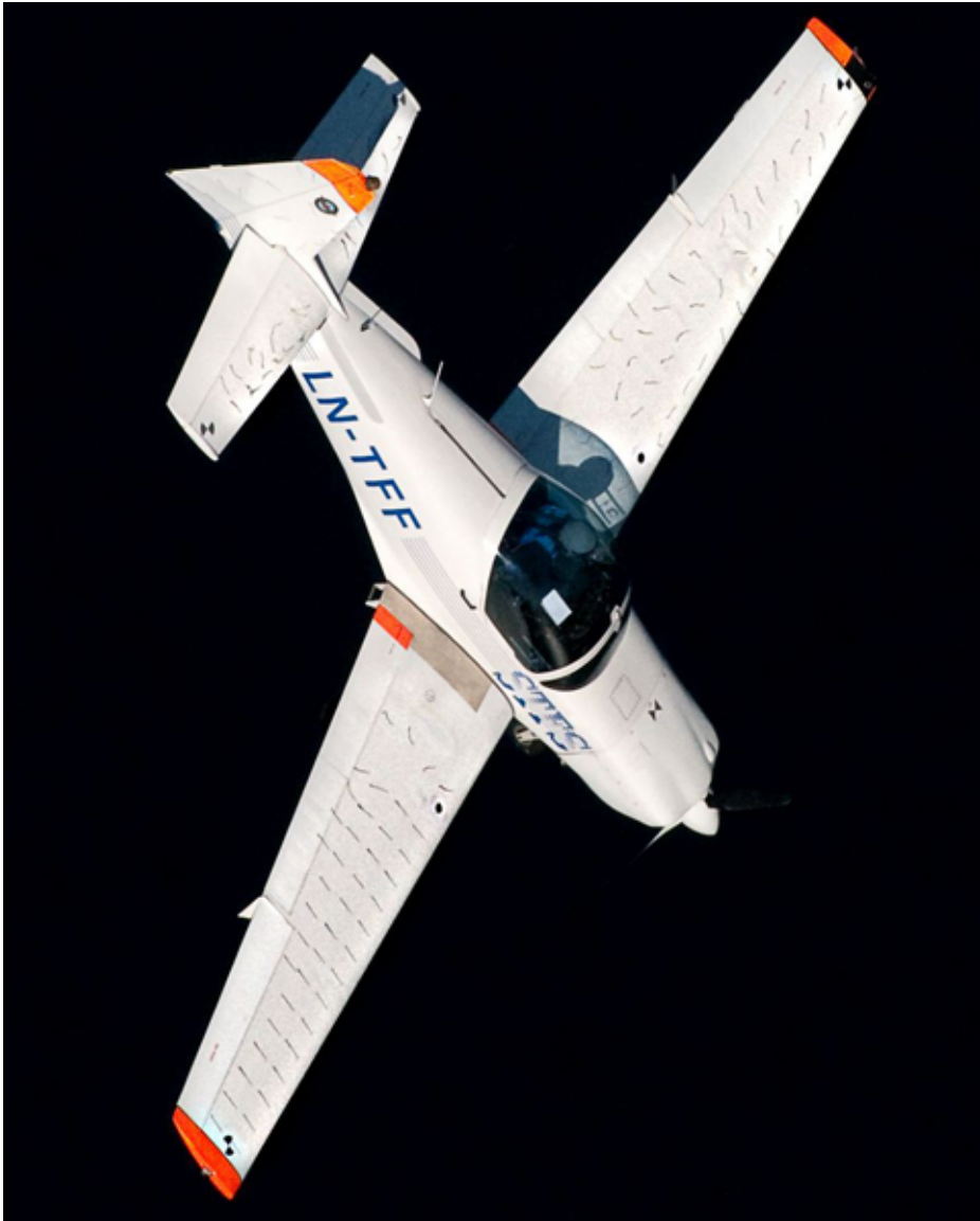
Figure 53. The aeroplane just before completing one turn with recovery controls set (the third turn from spin entry, left hand spin). All of the outside wing tufts indicate streamline flow. Flow on inside wing is still irregular at this point.
