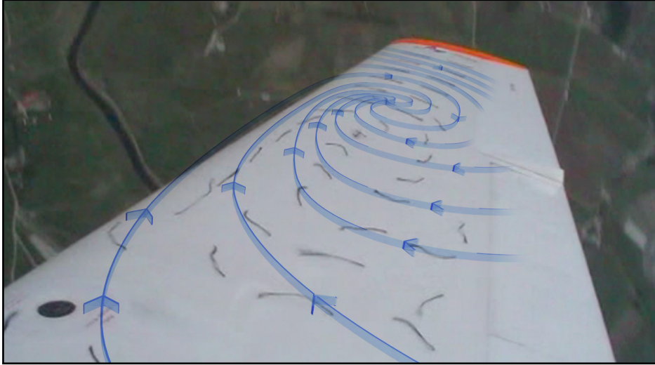
Figure 50. A large vortex forms on the outside wing as indicated by the wool tufts. The blue lines are drawn to illustrate how the shape of the vortex might be and arrows indicate flow direction.
