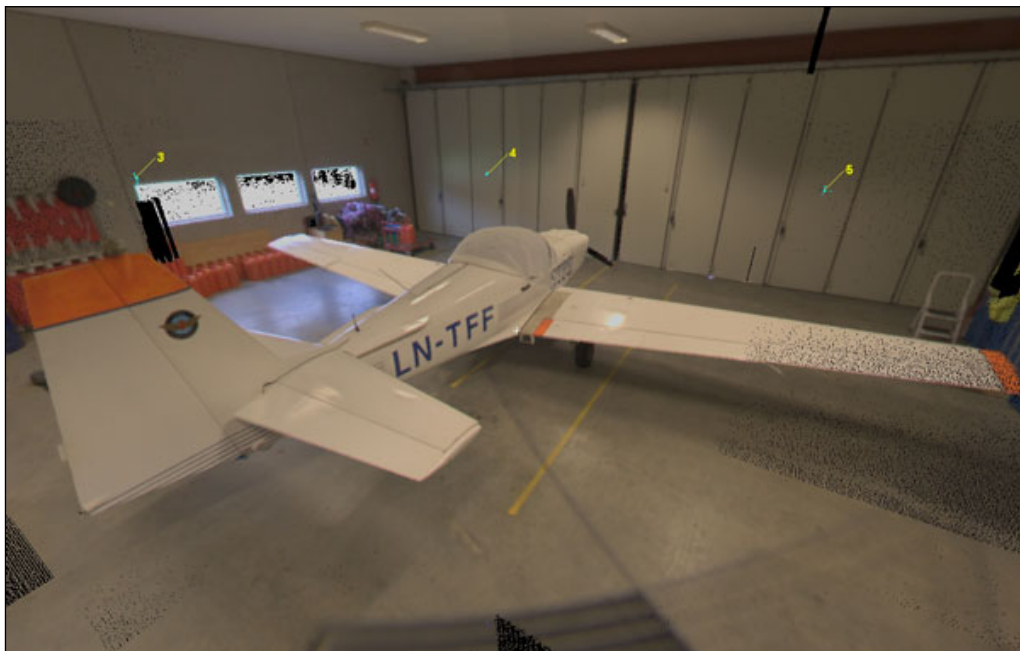
Figure 12. The coloured point-cloud of the Firefly. Note the laser scan targets on the walls.
