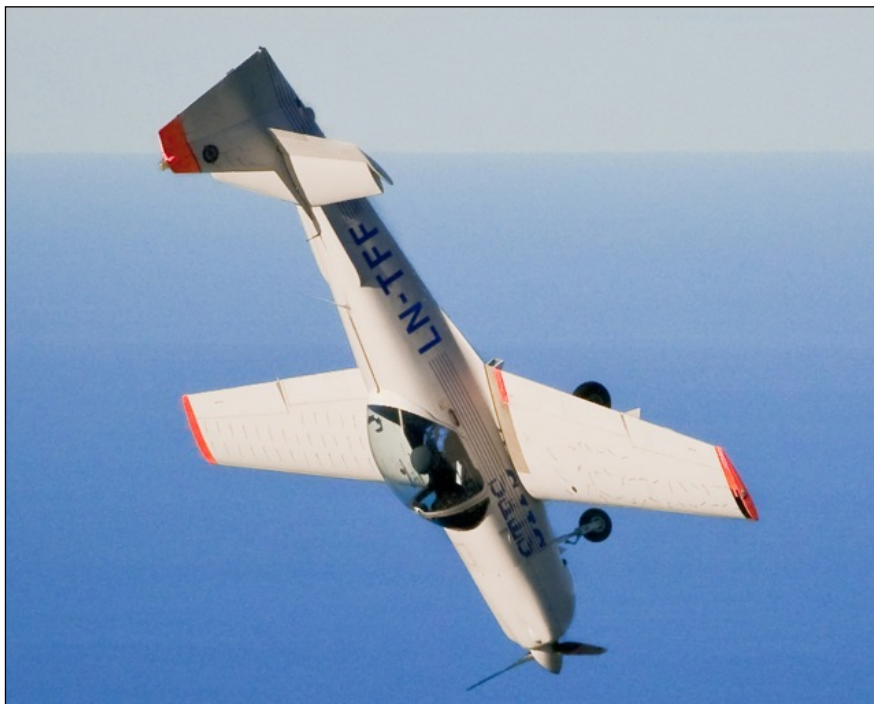
Figure 17. Left spin entry (just over \frac{1}{2} turn) ‘shot’ from the helicopter.
