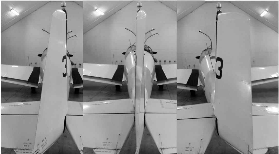
Figure 62. Pictures of the Safir rudder showing full left, neutral and full right positions. Note the twisted rudder and the difference in rudder angle when displaced full left and full right.
