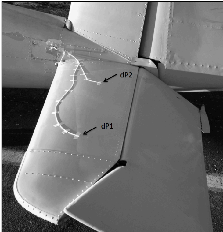
Figure 27. The modified Pitot-Static system circuit board was installed in the aft Saab Safir fuselage and the plastic tubes were routed on upper and lower surface to the desired points used for measurement.
