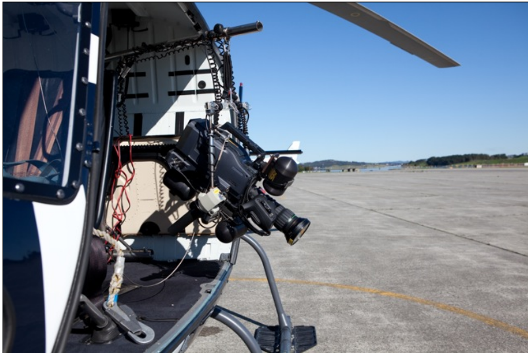
Figure 15. The camera installation in the helicopter.
