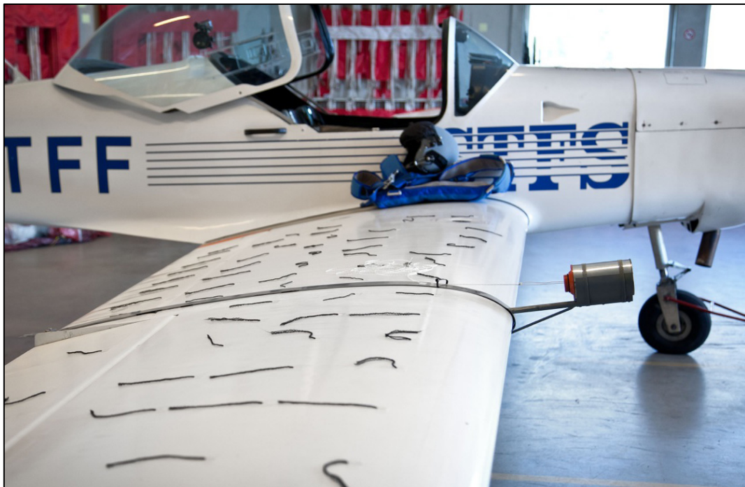
Figure 30. The ‘smoke boom’ attached to the right wing of the Firefly research aeroplane.
