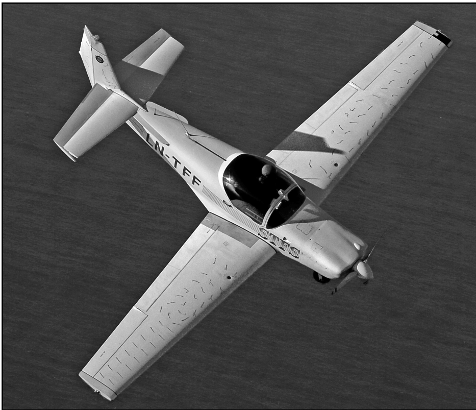
Figure 51. Tufts on the wing at just past the \frac{3}{4} turn in a left hand spin. The vortex on the outside (right) wing is clearly seen where the flap meets the aileron.
