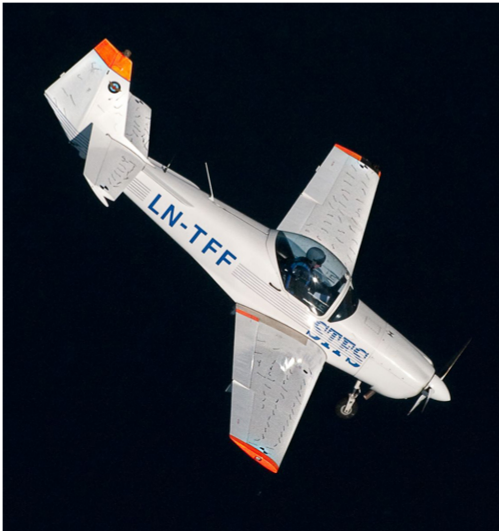
Figure 52. At the 2-turn point, spanwise outboard flow is clearly apparent on the outside wing. Only the outer row of tufts are streamline. Irregular flow can be seen on the inside wing.
