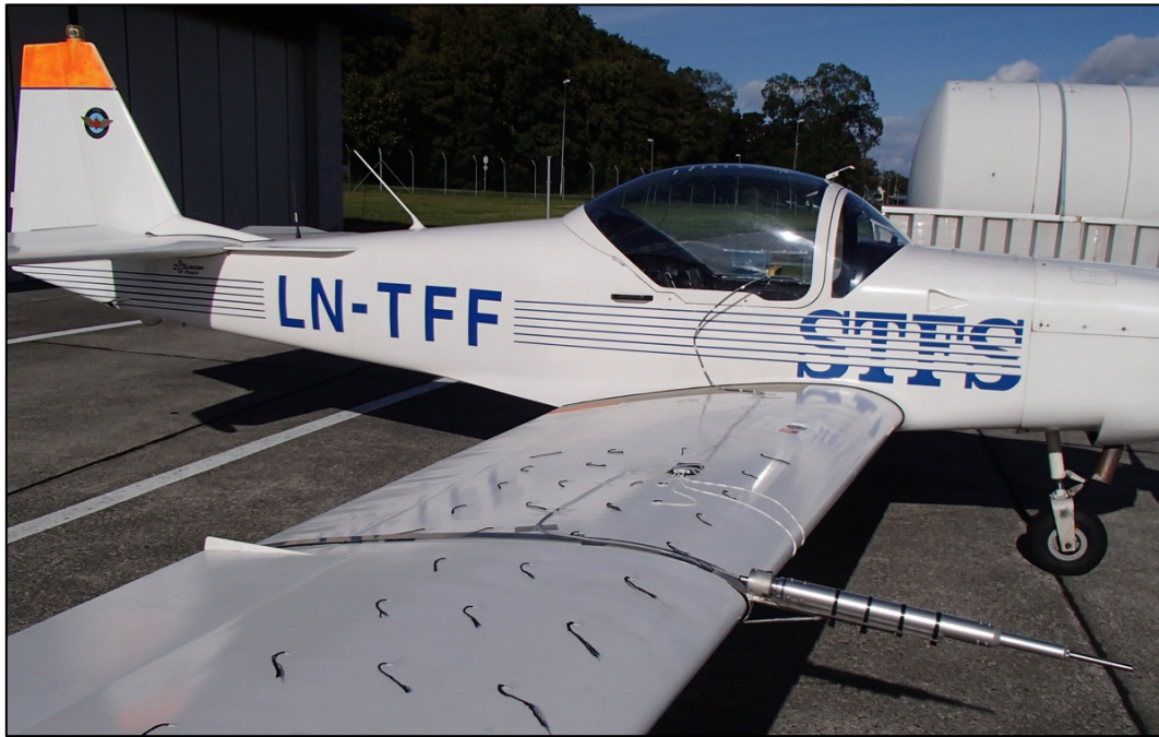
Figure 31. The ADP attached to the right wing of the Firefly research aeroplane. Note the negative incidence of the ADP relative to the wing chord.
