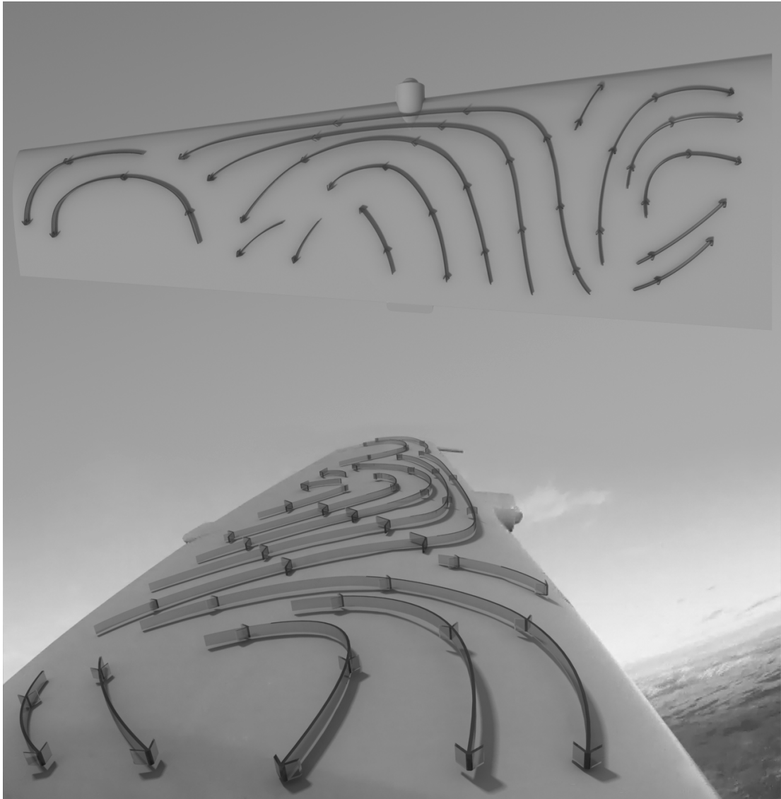
Figure 64. Illustration based on the flow direction indicated by tufts, showing the dipolar vortex structure temporarily observed on the outside wing of the spinning Safir after the 1-turn point in the right spin.
