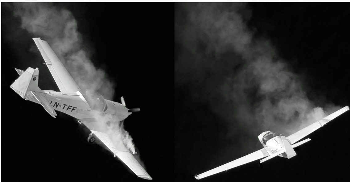
Figure 60. Before the 2-turn point (left image) in the spin, and after full right rudder was applied for the recovery at the 2-turn point (right image), smoke was visible towards the wing tip.
