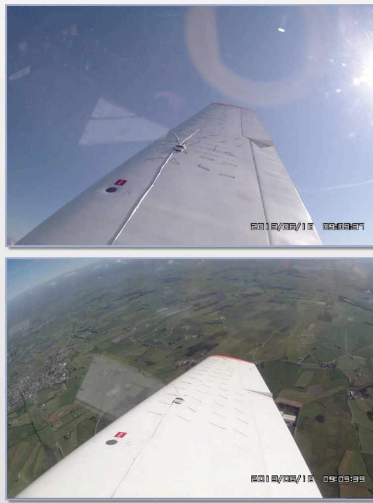
Figure 71. The high- and low-wing positions during the post-stall LAR motion.
