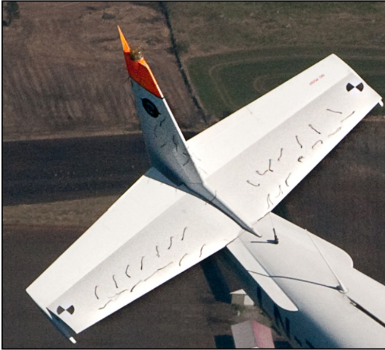
Figure 56. The tufts on top of the stabiliser indicate the presence of a leading edge vortex.
