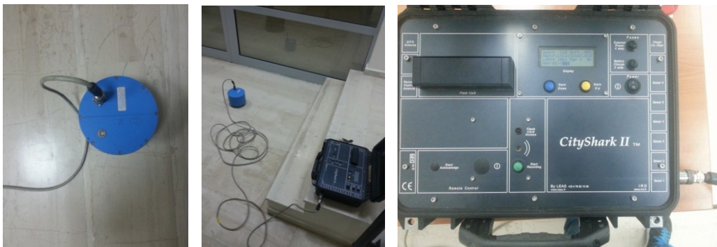
Figure K.3. Instrumentation for ambient noise recordings
