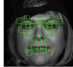
Fig. 6 Example of a normalized face image with highlighted regions from which the features were extracted
