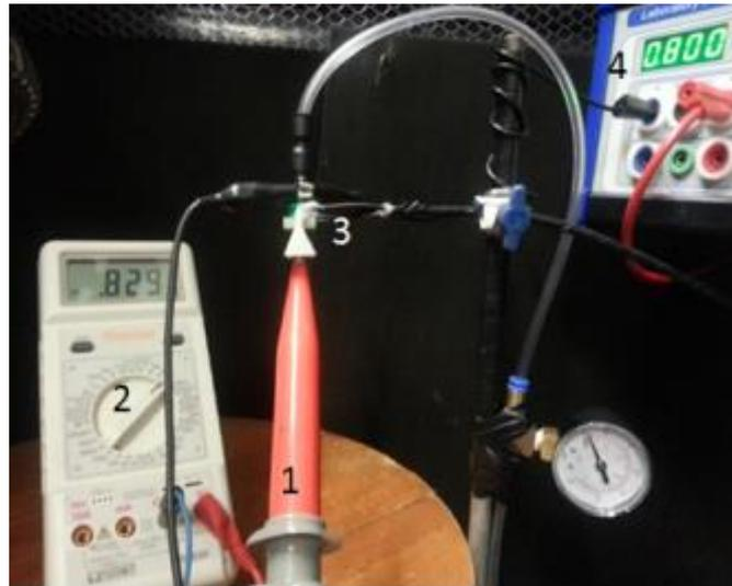
**Figure 6.17: Checking the induction voltage on the nozzle electrode. High voltage prop (1), multimeter (2), induction nozzle (3) and high voltage supply (4).**
