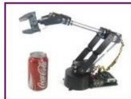
Image of AL5D Arm with optional wrist rotate.
