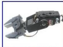
Gripper with Wrist Rotate.
