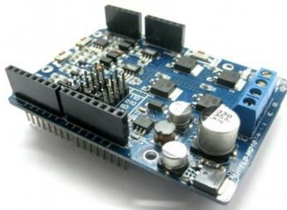
**Figure 5.8: The Cytron MD-10 DC motor drive shield [106].**
