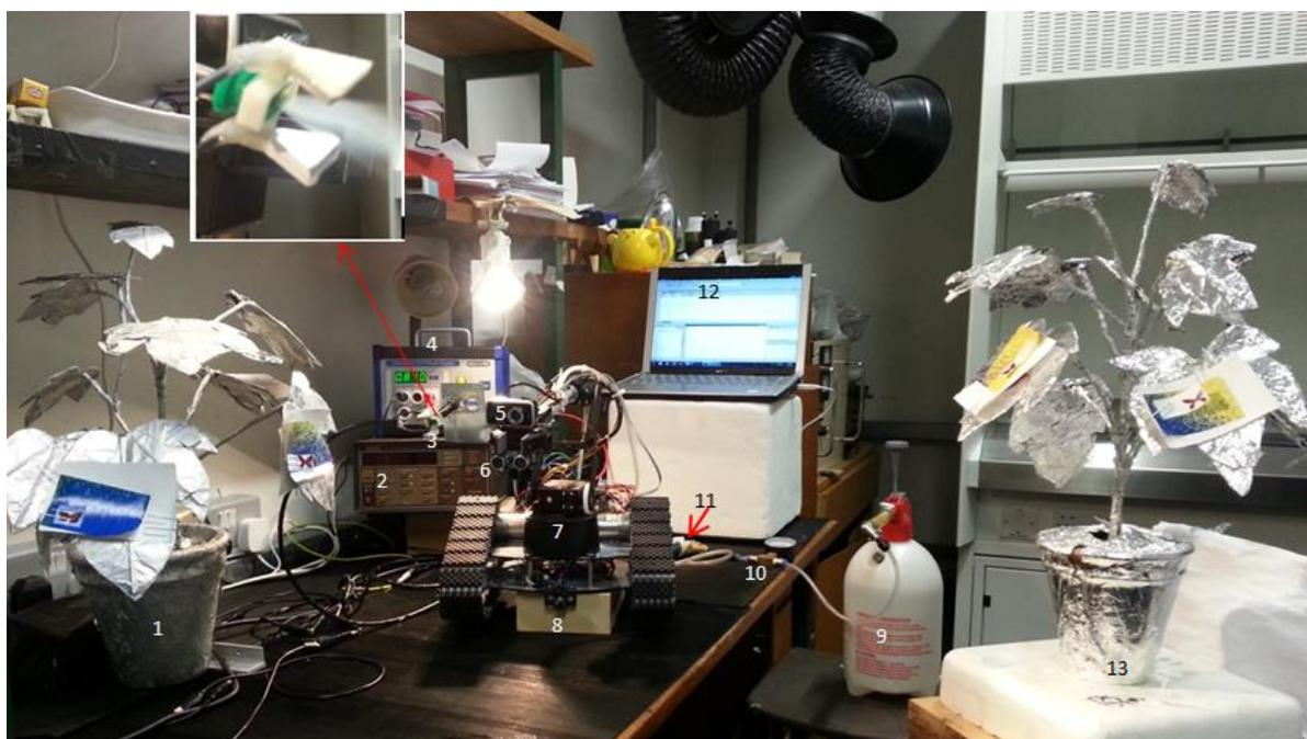
**Figure 6.9: The components of the experimental setup: artificial cotton plant with the targets (1), electrometer (2), induction nozzle (3), high voltage supply (4), CCD camera (5), sensor for measuring nozzle to target distances (6), robot (7), sensor for searching plants lines (8), water bottle (9), air pressure gauge (10), solenoid valve (11), personal computer (12) and, artificial plant (13).**
