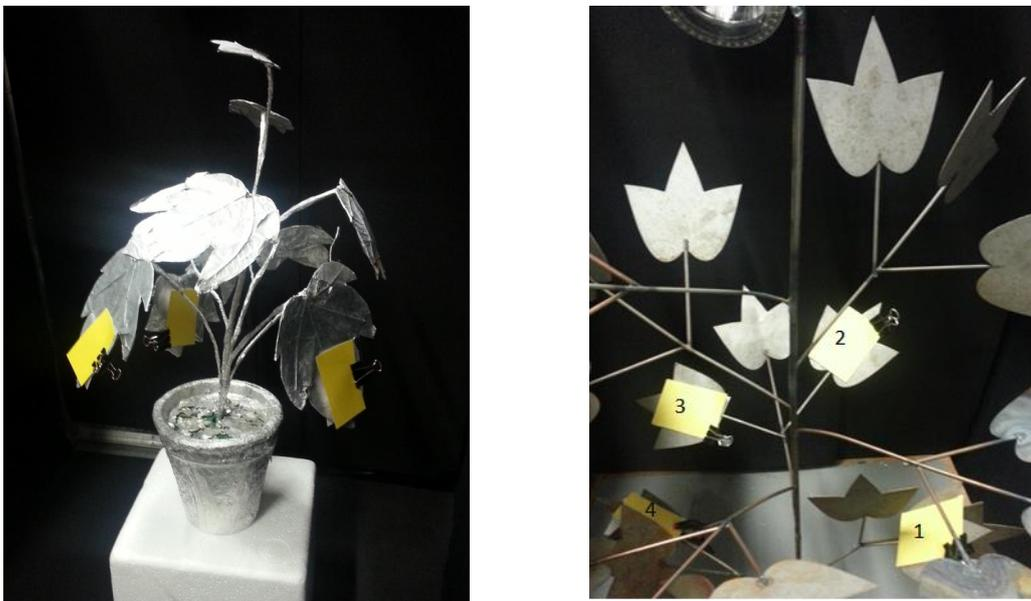
**Figure 3.26: Artificial plants inside the Faraday pail with water sensitive paper on the top and bottom surfaces of the leaves (1,2,3, and 4).**
