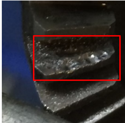
Figure 5-15: Seeded defect on the pinion tooth.
