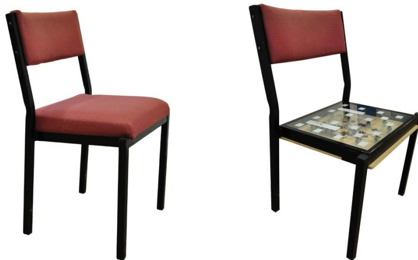
Figure 5.1 – Standard office chair converted to DTS chair by modifying the seat to distributive surface with distributed underneath sensing elements.
