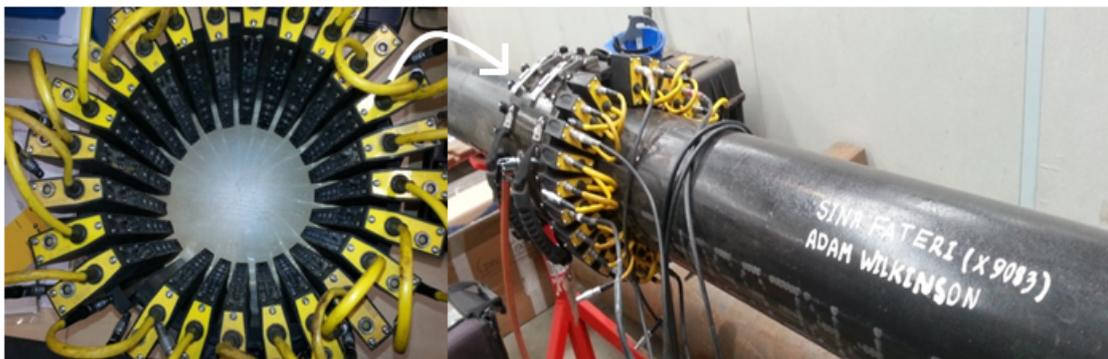
Figure 6.26: Phantom Teletest collar tool (left) and coupled to the 6 schedule 40 inch pipe (right)
