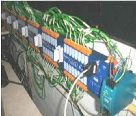
(a) Data scan module of gas cooler test rig
