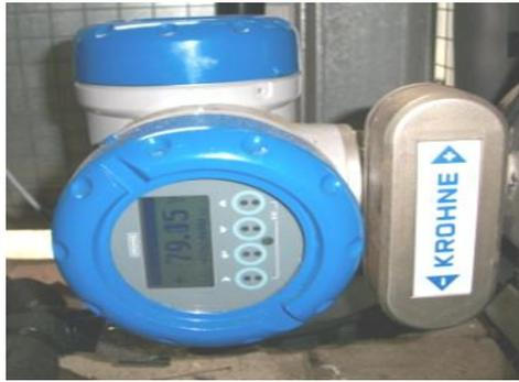
**Figure 3.24 Flow meter Optimass-3000-S03**
