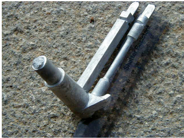
Figure 3. Photograph of the rheomoulded AZ91D alloy component.
