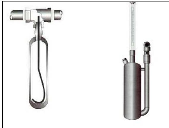
Figure I.3, Wick odorizer, adjustable and non-adjustable, source: (Tenkrat, et al., 2010)
