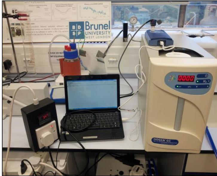
Figure 3.17, Experimental Setup of the PEM Electrolyser
