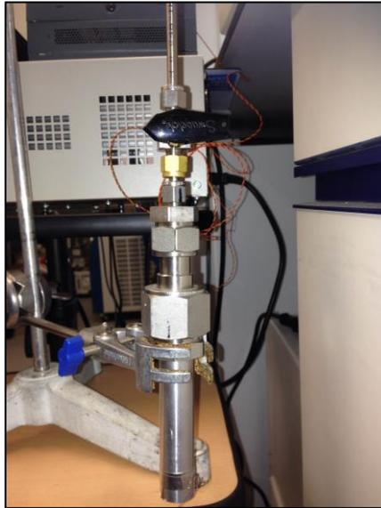
**Figure 3.14, Metal hydride storage tank**
