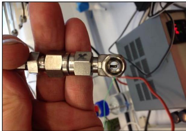
**Figure 3.15, Thermocouple for the measuring of the temperature of the PEM electrolyser produced hydrogen**
