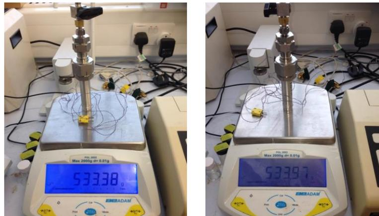
**Figure 4.17, measurement of the weight of the Metal Hydride tank at the beginning and at the end of the experiment**
