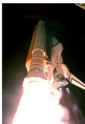
**Figure I.5, Space shuttle launch, blue colour for H<sub>2</sub>-O<sub>2</sub> fuelled engines, source: (NASA, 2013)**
