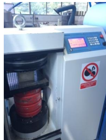
Figure 3.9 Compressive strength test of prism (Left) and cube (Right)
