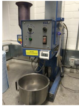
(a) Mortar mixer
