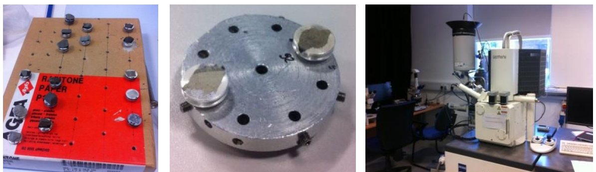
Figure 3.13 Samples on pins (Left), samples on SEM disc (Middle) and SEM machine (Right)
