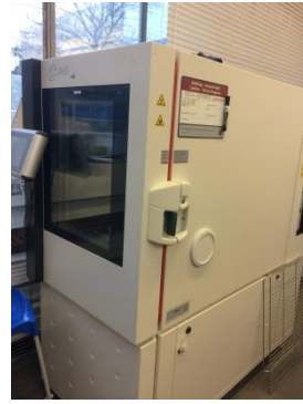
(e) Temperature-controlled unit
