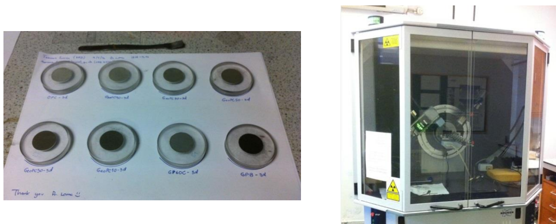
Figure 3.11 Sieved particles in XRD testing discs (Left) and XRD machine (Right)
