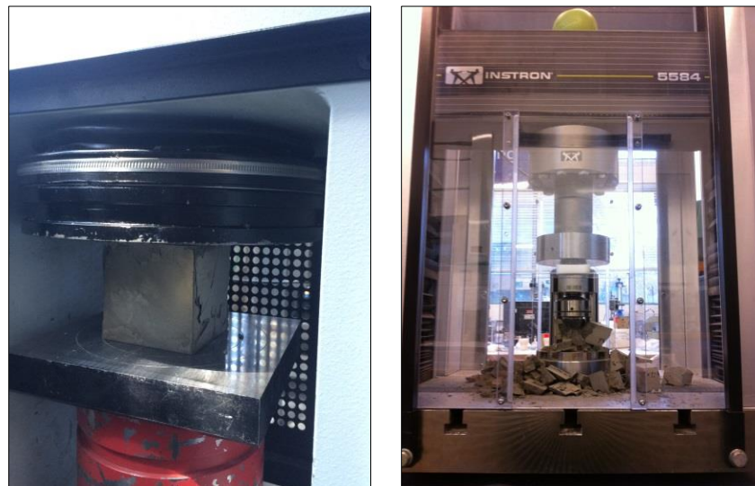
Figure 8.2 Compression test of cubic sample (Left) and prismatic sample (Right)
