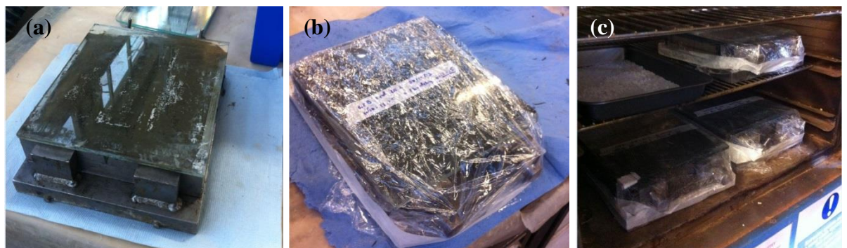
Figure 6.1 (a) Casting, (b) Moisture loss protection, and (c) Under curing regimes
