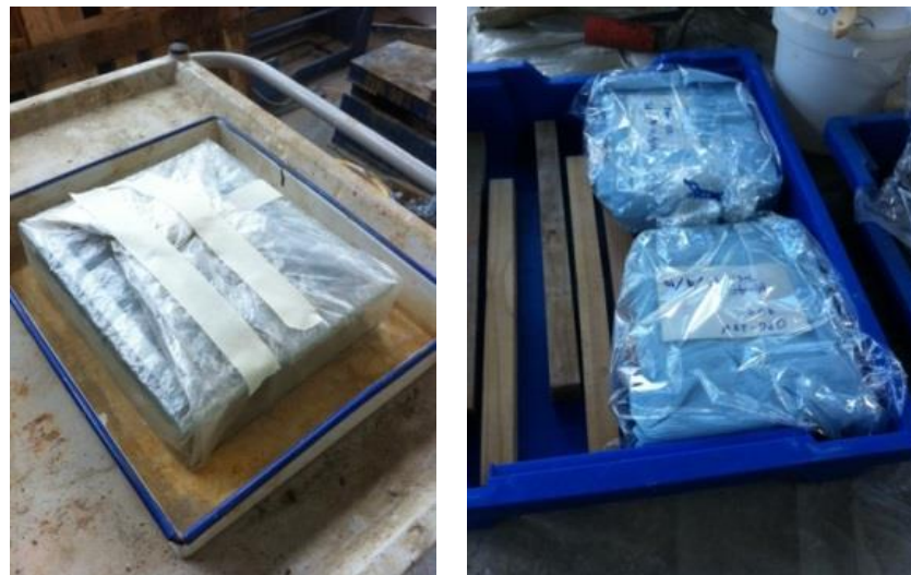
Figure 3.6 Samples wrapping after casting (Left) and placing in plastic bags before curing (Right)
