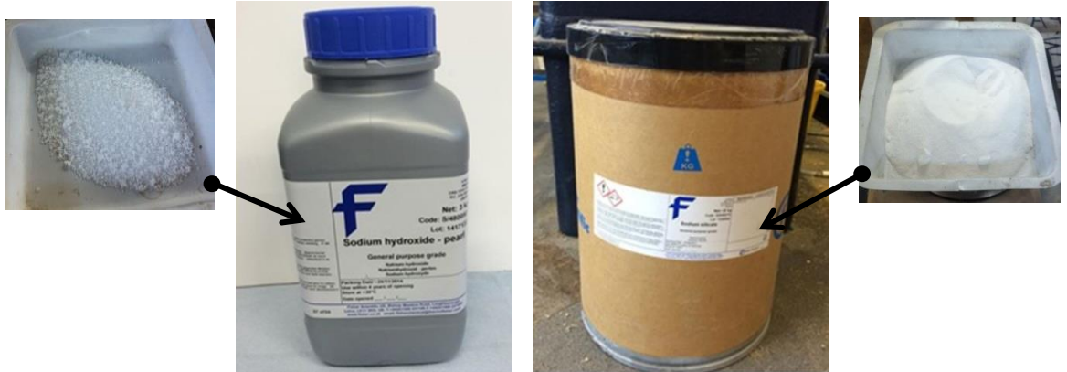
Figure 3.4 Sodium hydroxide (left) and sodium silicate (right) in containers
