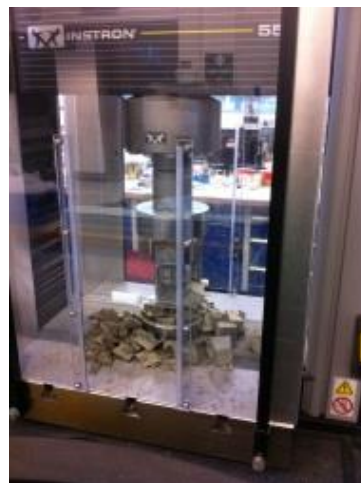
Figure 3.9 Compressive strength test of prism (Left) and cube (Right)
