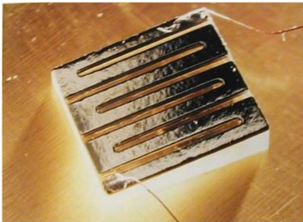
**Figure 4-1 InSb detector mounted on a quartz substrate**
