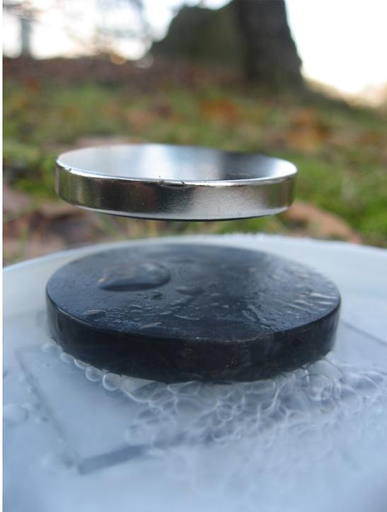
**Figure 3-1 Meissner Effect in action: A magnet levitating above Yttrium barium copper oxide ( $\text{YBa}_2\text{Cu}_3\text{O}_7$ ) cooled to  $-196^\circ\text{C}$  (Bobroff & Bouquet 2010)**
