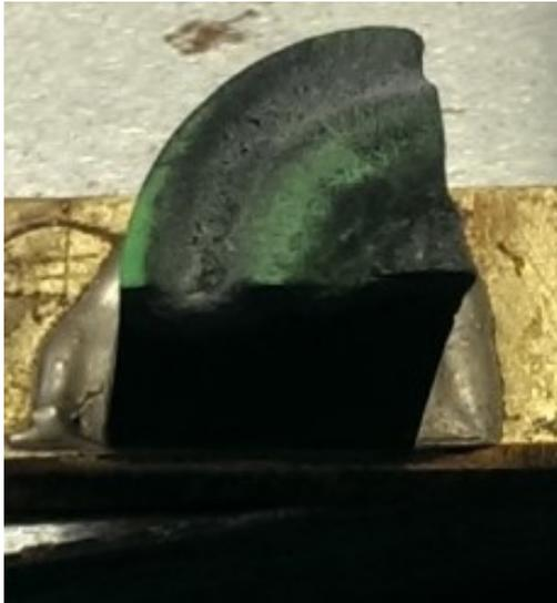
**Figure 3-12 GdBCO-Ag sample after ECM machining in 1.0 M NaCl**
