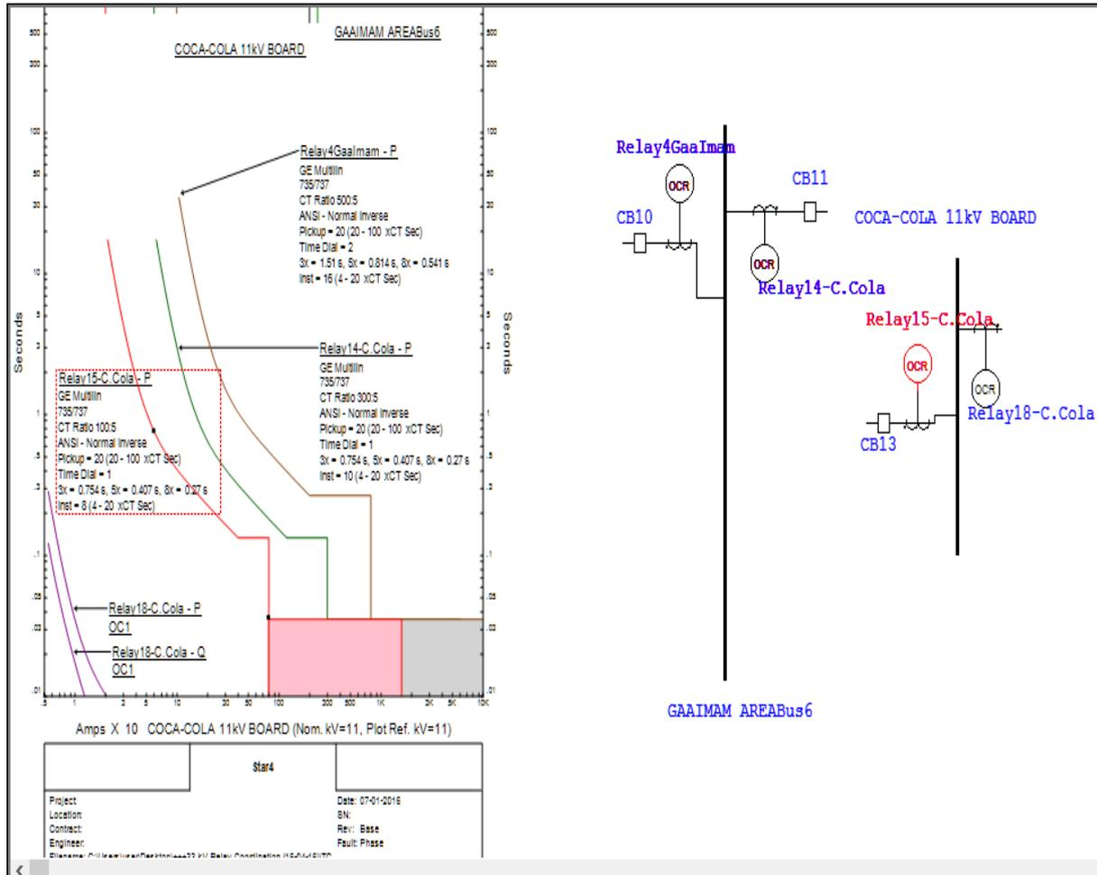
The intersection between TCC curves of the protection devices is the main reason for loss of coordination. There would be loss of coordination for feeders having crossings on TCC curves of main and backup protection devices. There would be mis-coordination at a particular level of short circuit current if the TCC curves cross.
