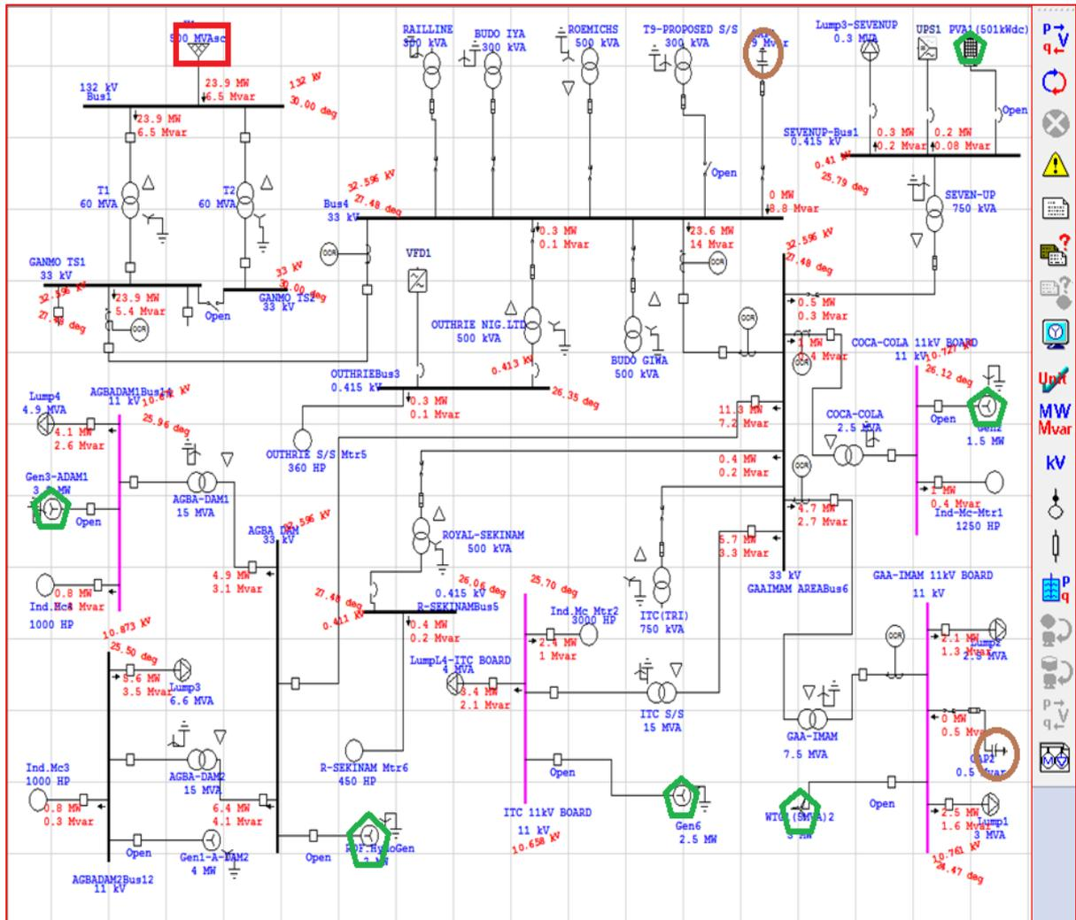
The swing or infinite bus was indicated in red square colour, the green polygons indicated the locations of the existing and proposed DGs, and the existing capacitors are in brown circles.
