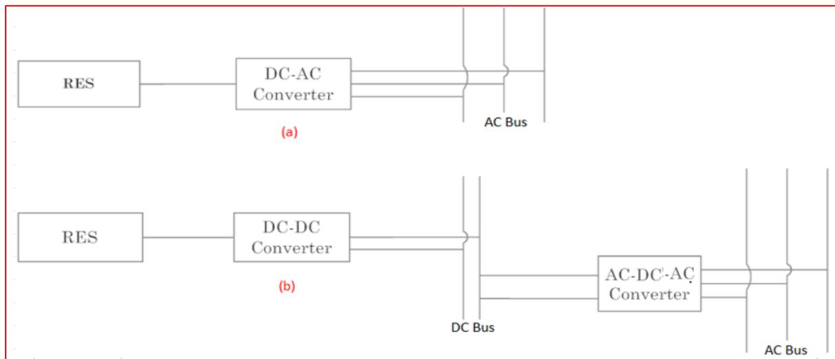
Figure 3.1. Interfacing methods of hybrid RES with the grid. 3(a). Direct conversion of DC-AC to the grid. 3(b). Interfacing with the DC and AC bus to the grid.
