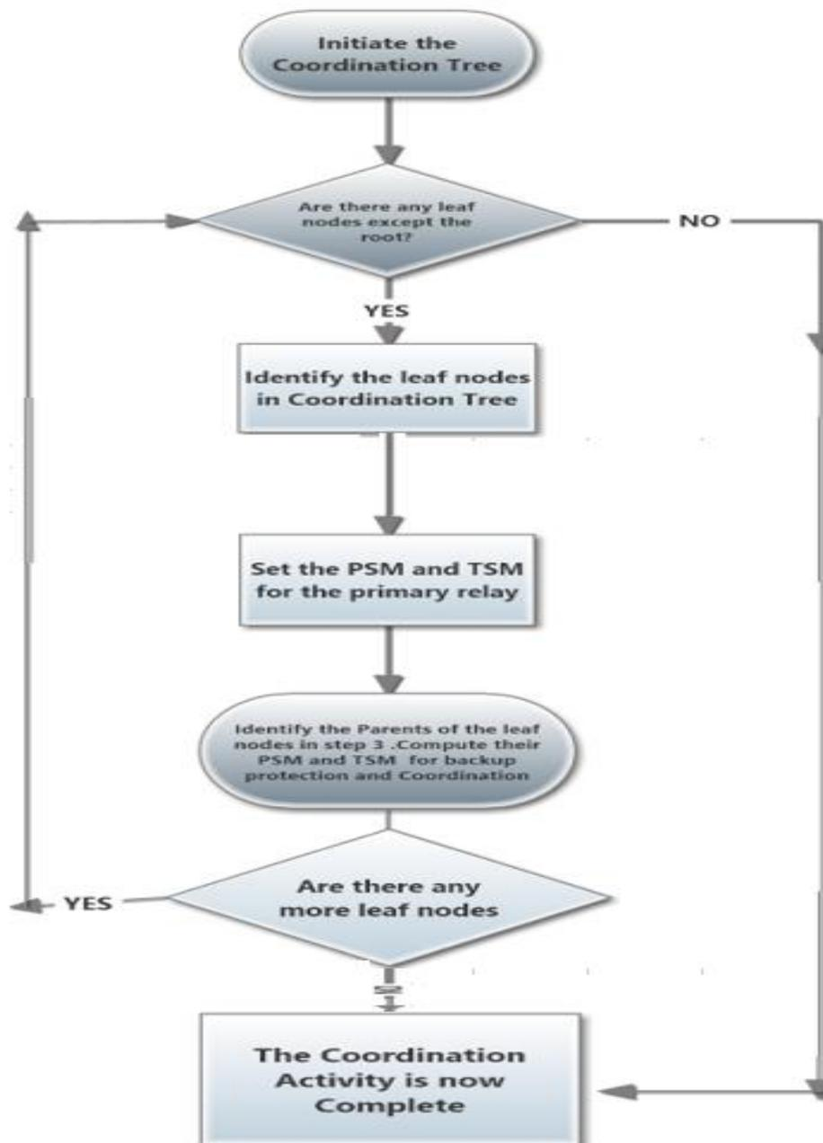
Figure 4.6 Proposed Leaf-Node Algorithm for Setting and Coordination of OCRs in a Radial System
