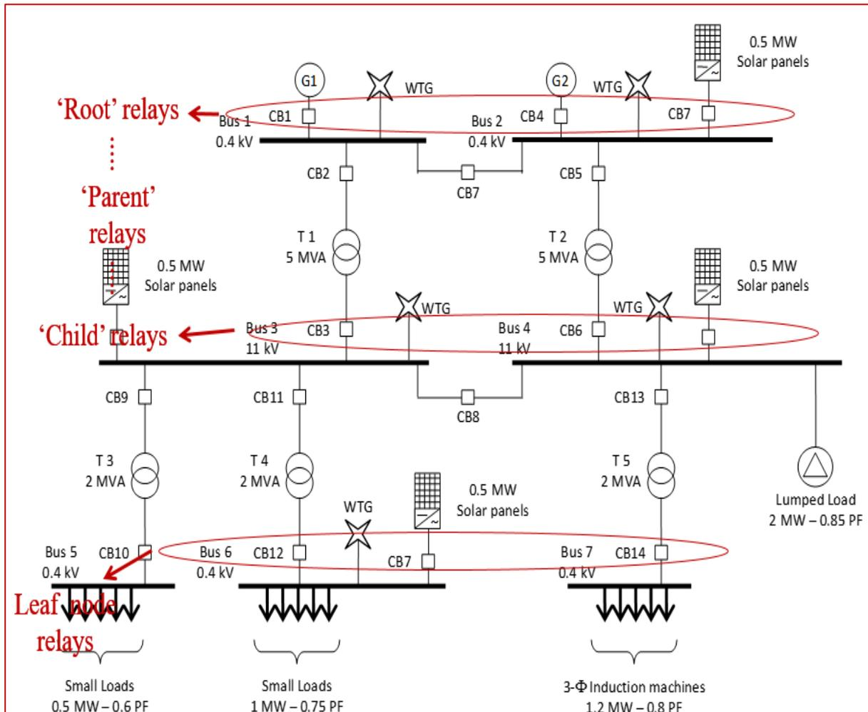
Figure 4.6 The Leaf-Node Algorithm as applied to Radial Distribution System
