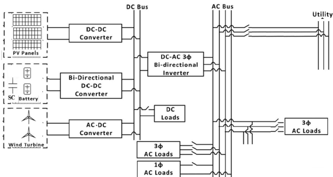
Figure 3.3 The HREDS configuration of the different converters and inverters
