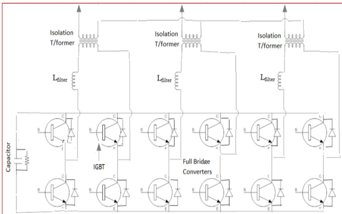
Figure 3.2: Schematic Diagram of DSTATCOM (Mitra & Venayagamoorthy, 2010)
