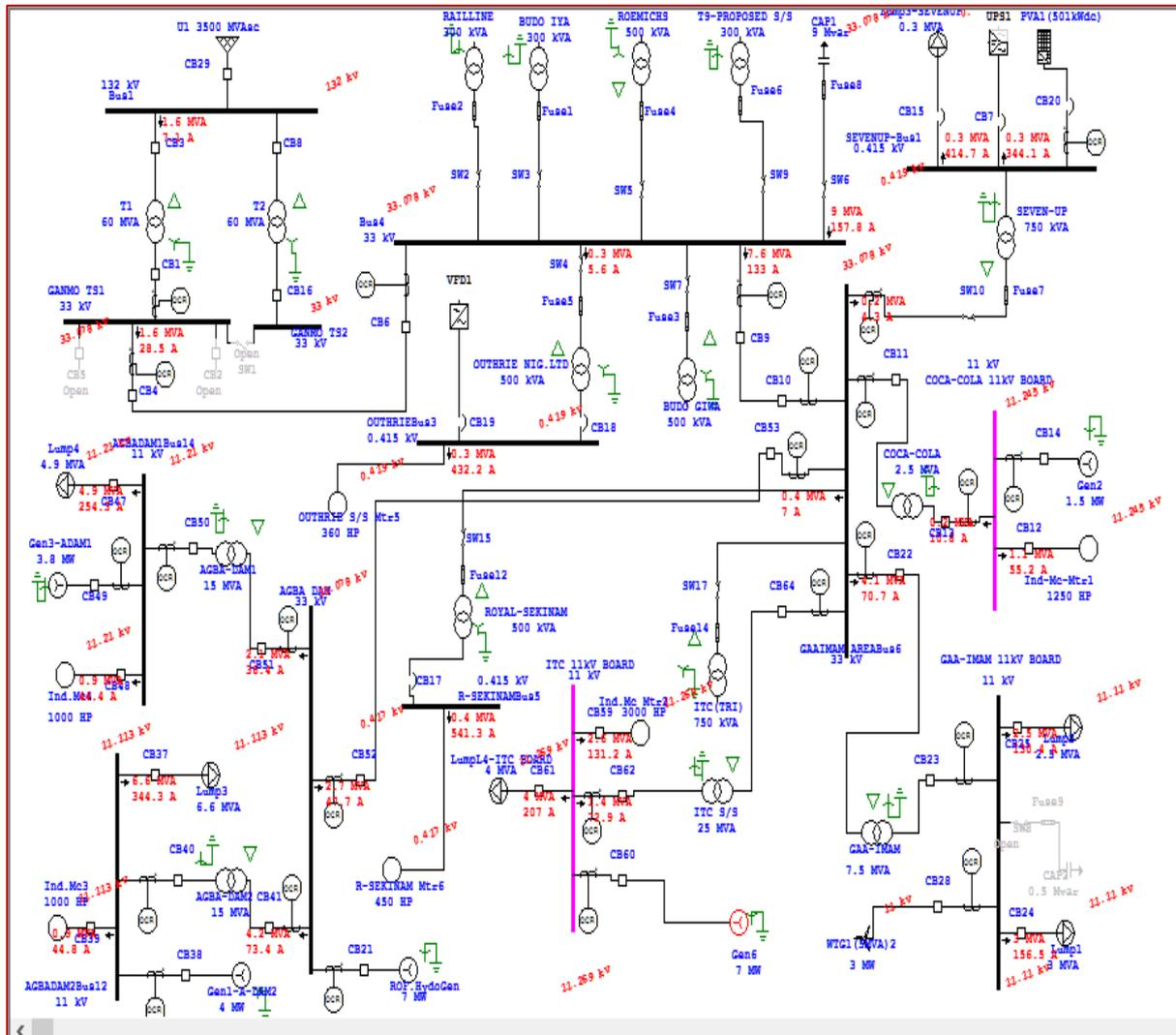
With DGs contributing nearly 100% of feeder load, the voltages at ITC 11 KV and the Coca-Cola 11 KV boards, had caused overvoltages at these buses, which could cause miscoordination at the respective OCR relays
