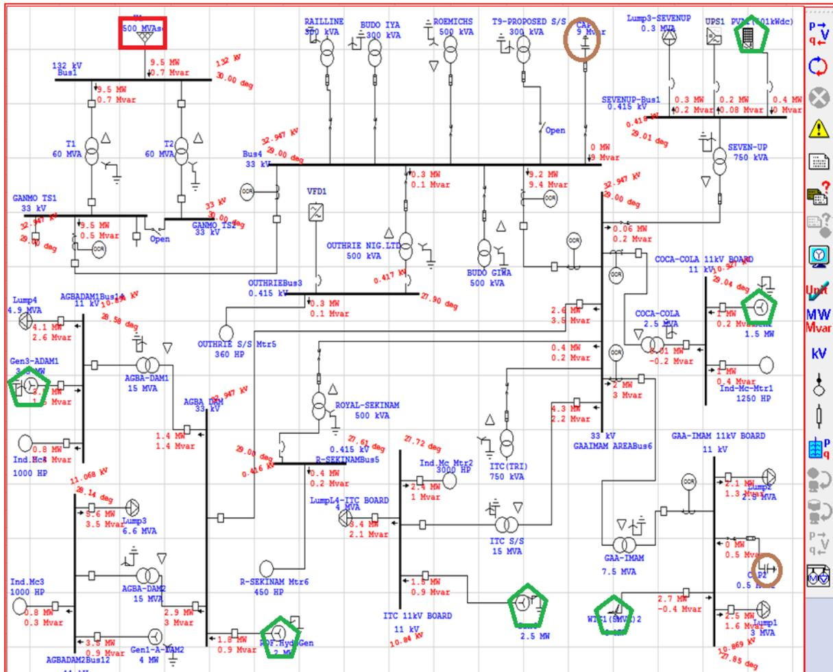
The penetration of more than 65% DGs amounted to transmission capacity relieve in the form of distribution capacity relief since there was a reduction of 14.4 MW (23.9 – 9.5), and 5.8 MVAR (6.5 – 0.7) when the DGs were included in the simulation. This reduction amounted to (24.77 – 9.53) MVA i.e. 15.24 MVA which was = 61.53%, which was supplied by the DGs.
