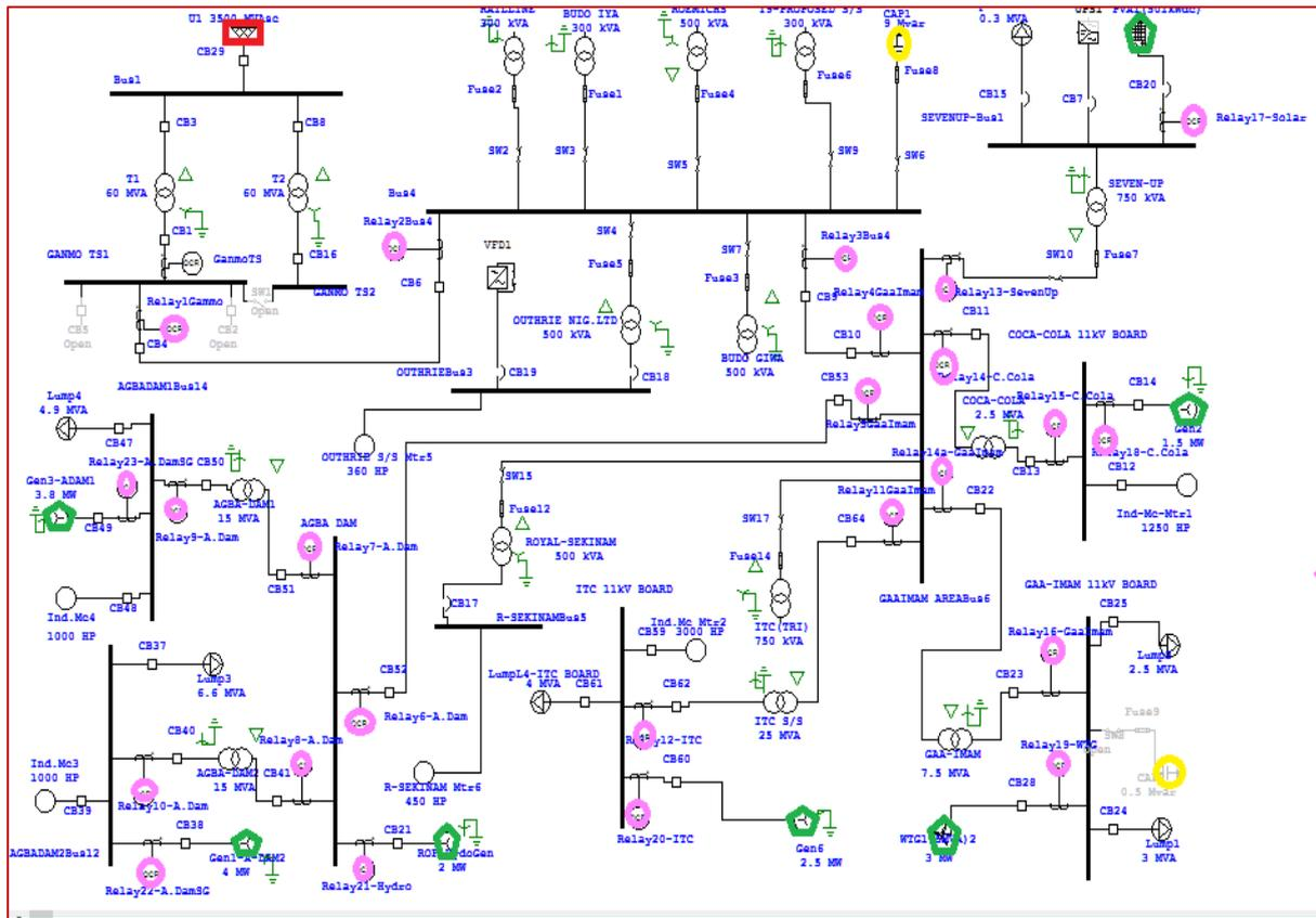
Figure 5.2 Study case circuit showing all the relays for coordination.
