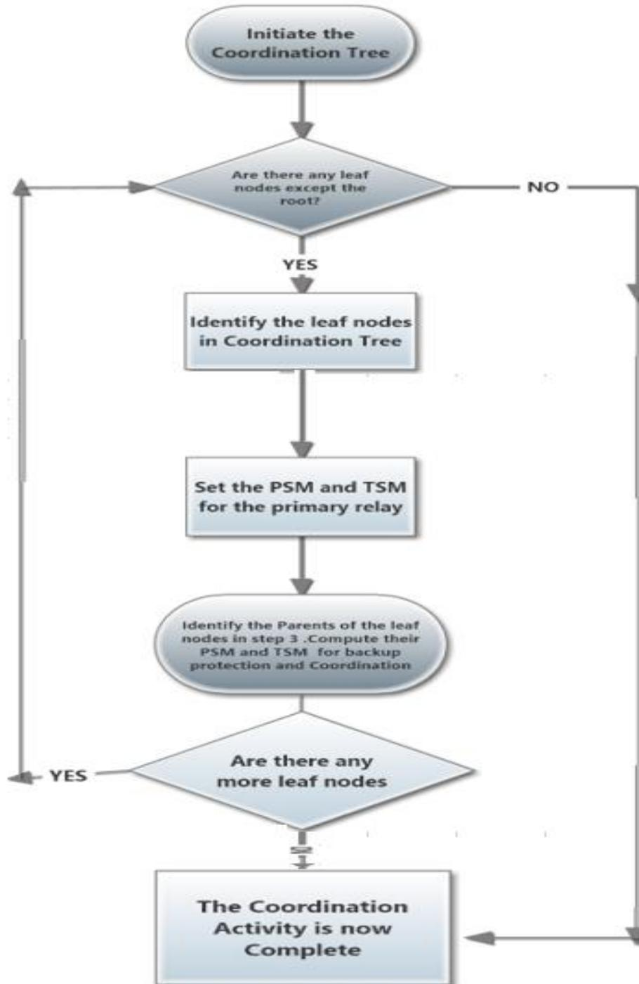
Starting the coordination from 'Leaf Node' relays to 'Child' relays, to 'Parent' relays and then finally to the source or 'Root' node relays, the PSM and TSM were calculated for each relay. The root node (parent relay) had no parent while the leaf-node had no child.
