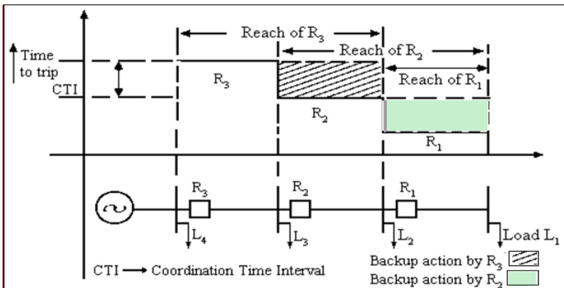
Figure 4.3. Overcurrent Protection Zones of Radial Distribution System (NPTEL - Electrical Engineering - Power System Protection Group, 2006)
