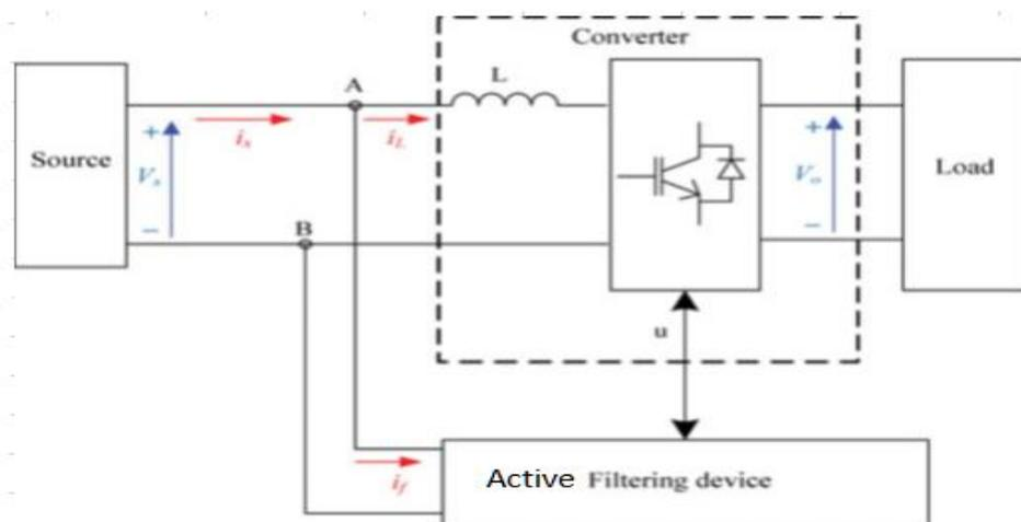
Figure 3.4 The filtering device for a DC-DC converter (Shahin, & et al, 2011)
