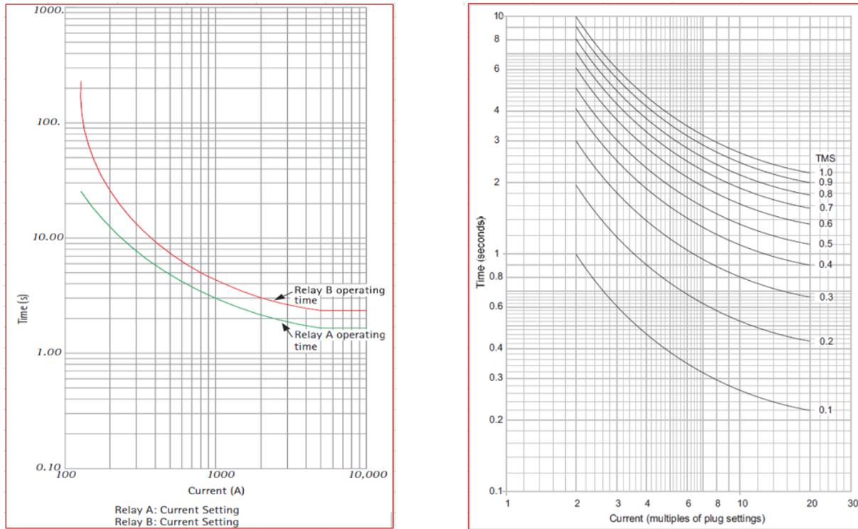
a) The characteristics of different relays. b) Typical multiples of pickup setting currents
