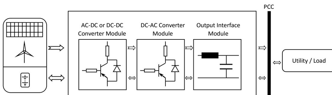
Figure 2.2 Generalised control design of PE interface
