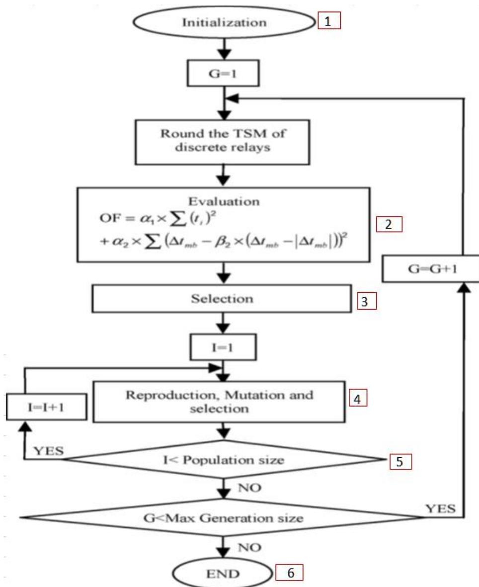
Figure 4.5 Flow diagram of GA application (Razavi, F; & et al;, 2008)
