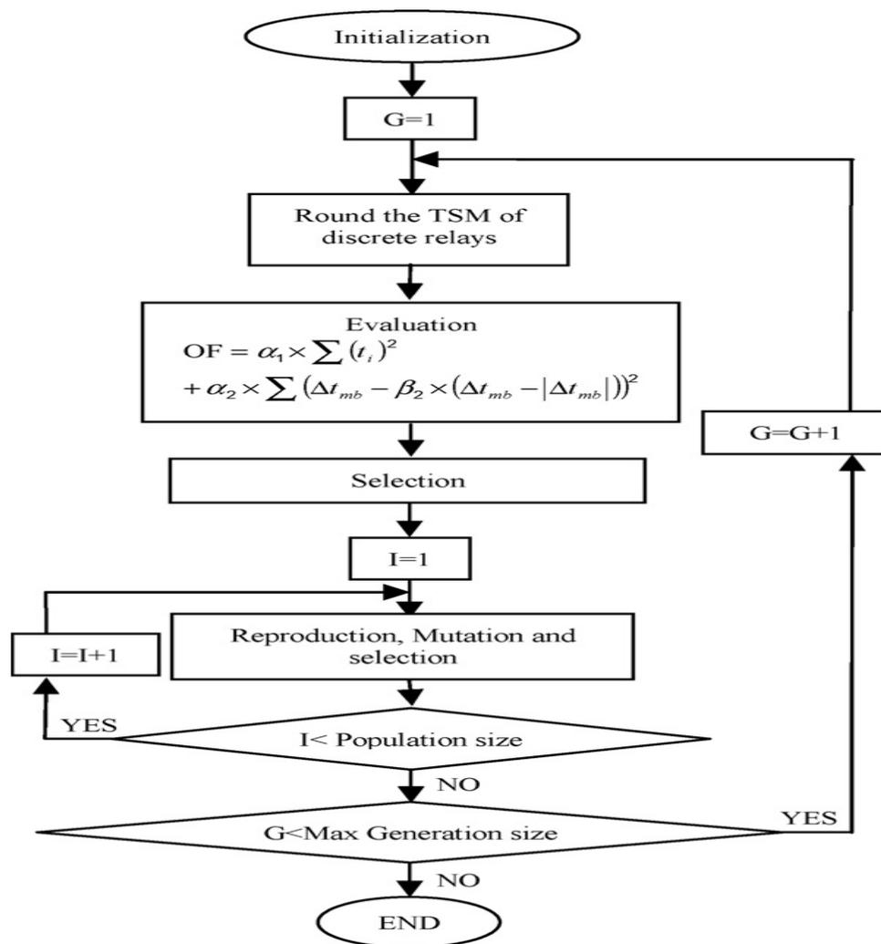
Figure 4.5 Flow diagram of GA application to relay coordination (Asadi & et al, 2008)
