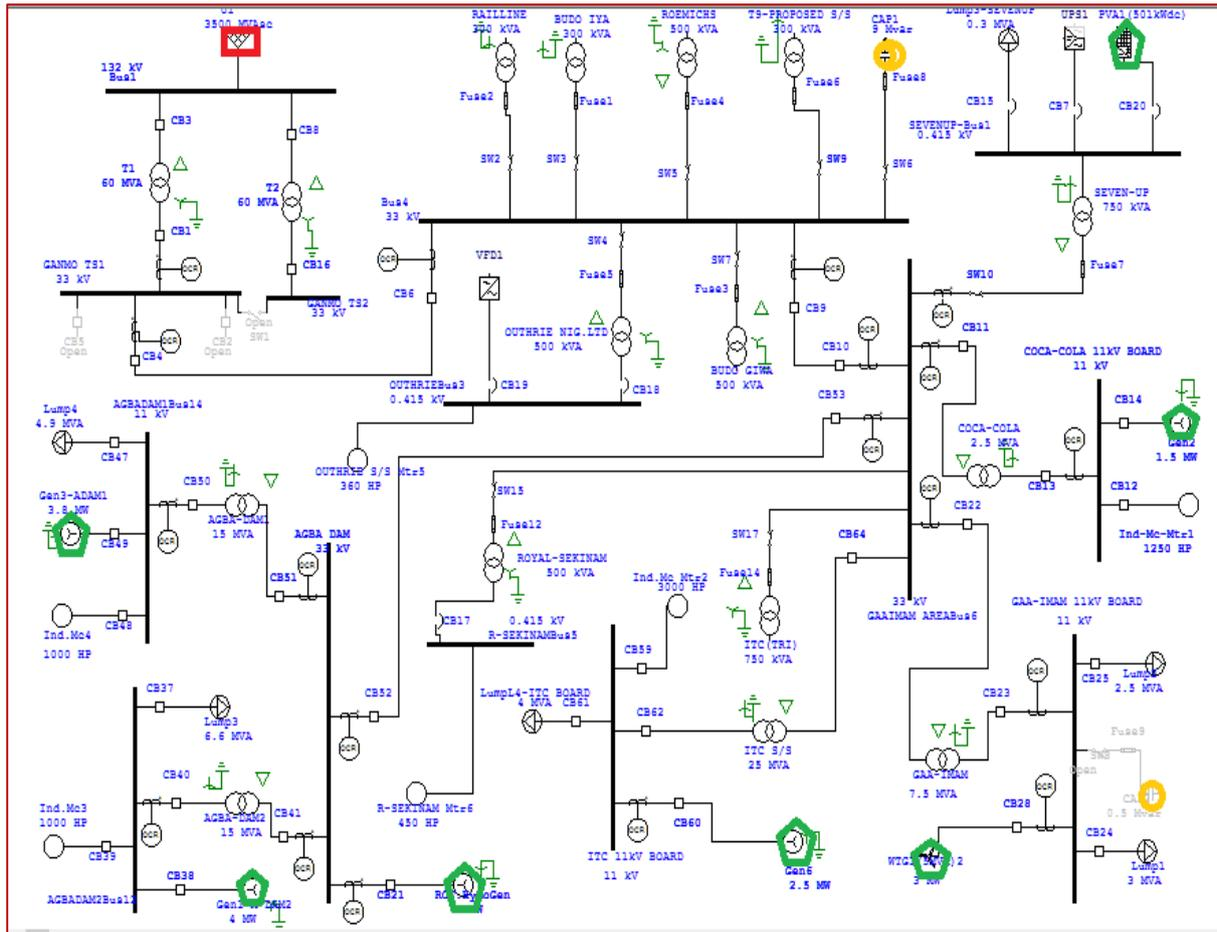
Figure 5.1 Case Study Distribution of Coca-Cola 33 kV Circuit (LFA)
