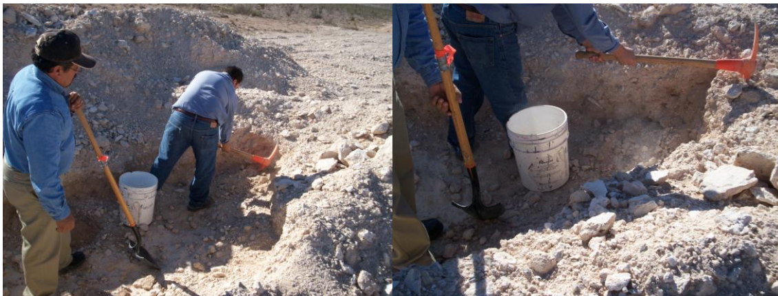
Photos 1 and 2. Sampling strata 1 composed of limestone sandy gravel conglomerate poorly sorted
