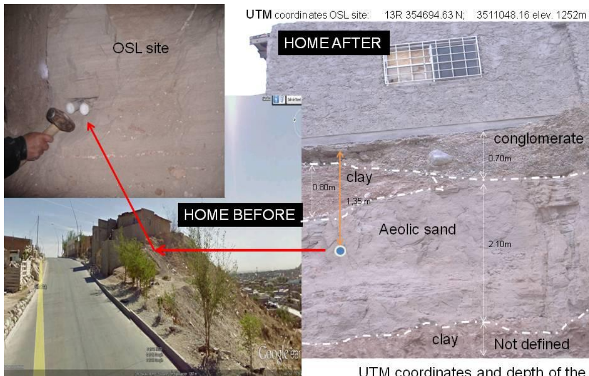
General location of the OSL sample of site P1 (see the home before and after and the Fig. 3.5A. OSL site location of collected sample (P1) Colorado Alluvial fan
