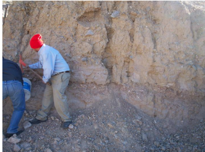
Photo 1 back to white home strata 3 flood of clay mixed with gravels and poor sorted pebbles of 1 inch to 3 inches diameter layer of 2.00 m.
