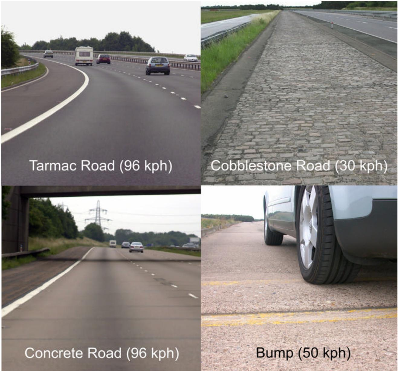
Figure 3 Road surfaces which produced the steering wheel acceleration time histories used in the laboratory experiments.
