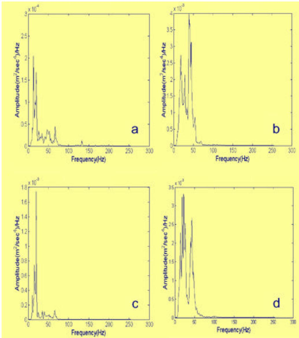
Figure 5 Acceleration power spectral densities of the steering wheel tangential direction acceleration time histories.
