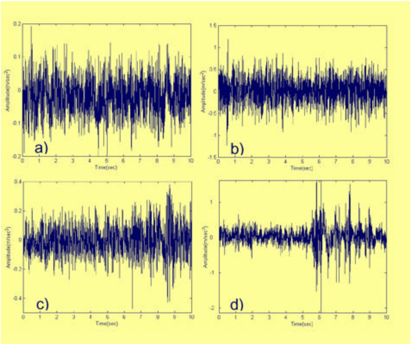
Figure 4 Steering wheel tangential direction acceleration time histories used in the laboratory experiments.
