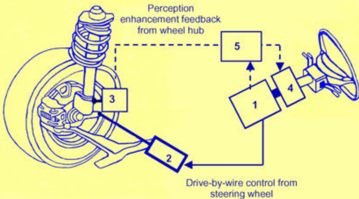
Figure 2 A perception enhancement system for by-wire steering.
