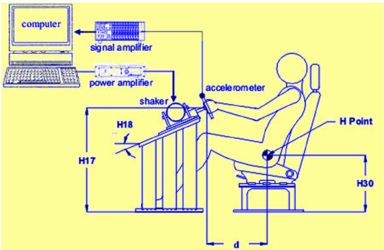
Figure 6 Steering wheel rotational vibration test simulator.
