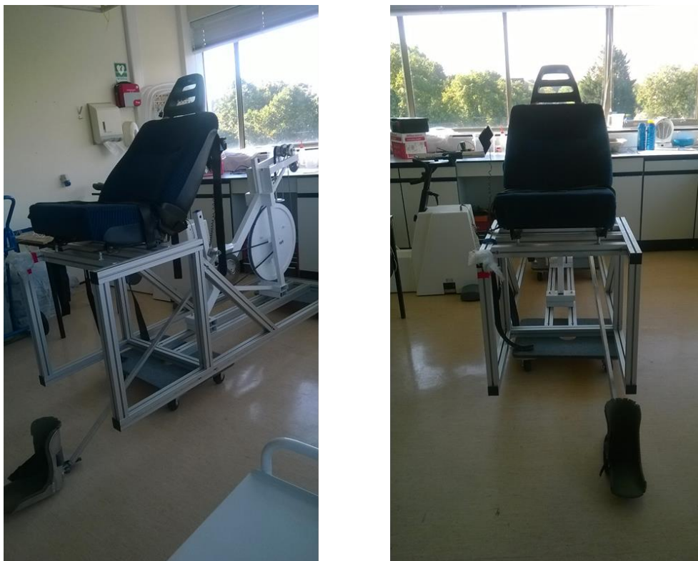
Figure 6-3. Modified Monark ergometer used for the dynamic knee extensor exercise protocol in study 2.
