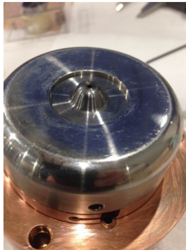
Figure 7.9 - Forward bump diaphragm plate manufactured according to design from Opera-2d simulations
