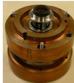
Figure 5.15 - Plasma chamber with magnets and magnets holder
