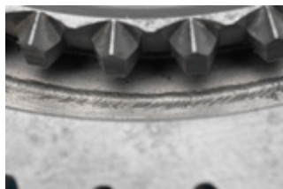
Figure 2.13 - Example of an EB welded gear cluster
