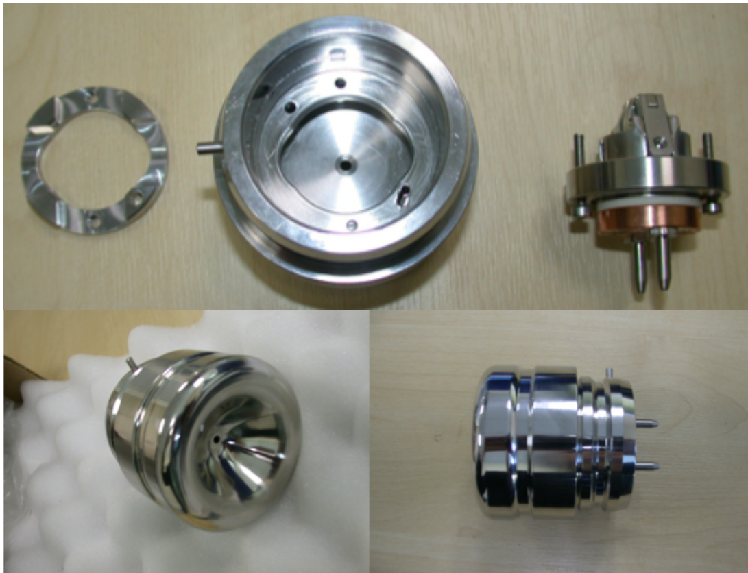
Figure 3.10 - Filament holder assembly and grid cup (top), and the filament holder accommodated in the grid cup (bottom)
