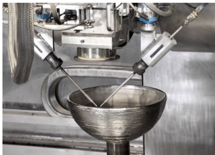
Figure 2.15 - Additive manufacturing using wire feed in titanium (Sciaky Inc. 2015)
