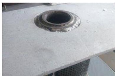
*Figure 3-4 Top of the DC simulator, where the melt is poured into.*
