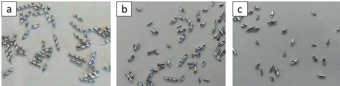
*Figure 7-7 Photographs of the chips obtained during machining for the extruded and heated bars of the following casts: (a) reference untreated cast, containing Al-5Ti-B(b) containing Al-Ti and Al-B, heated to 860°C, sheared and (c) heated to 860°C, sheared.*
