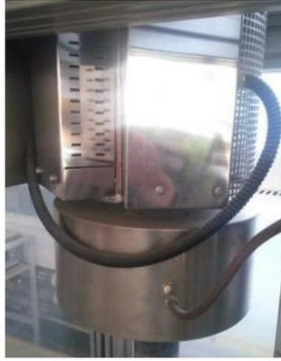
*Figure 3-5 Picture of the heating elements in which the steel mould is inserted and cooling water chamber.*
