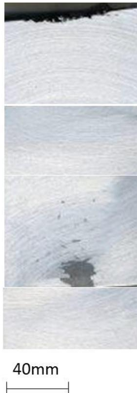
*Figure 4-12 Macro etched section showing the Pb segregation towards the centre of the billet for an Al-3Pb billet.*
