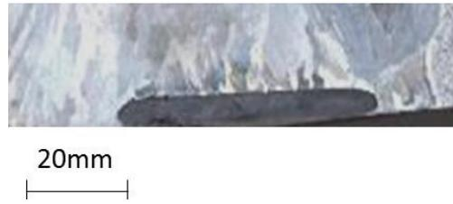
Figure 4-6 Macro etched section showing the bottom of DC simulator non sheared billet.
