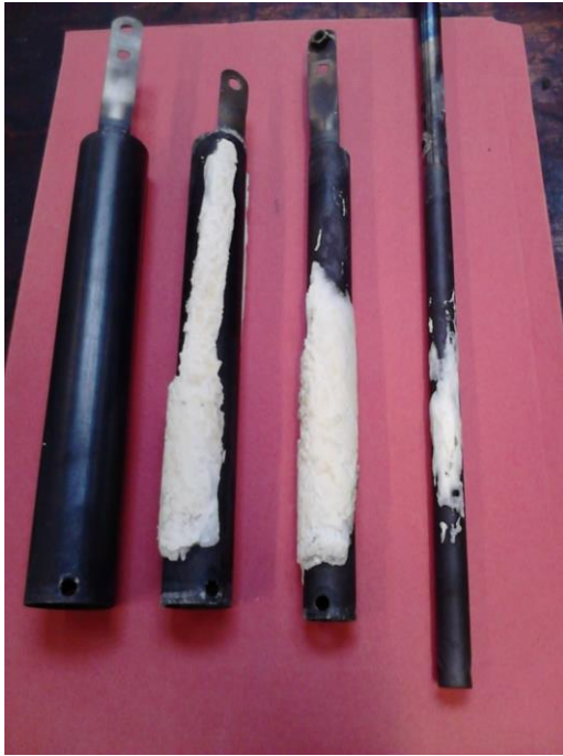
Figure 4.18: Photograph of the scaled electrodes after use at 8 V.
