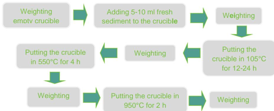
Fig. 3.8. LOI process in order to measure water content, calcium carbonate and organic matter
