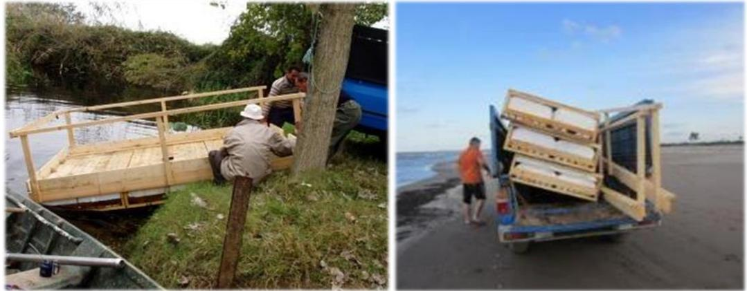
Fig.3.5. Portable and light weight coring platform built to take cores in lagoons using the Livingstone corer. (Photos: the Author)
