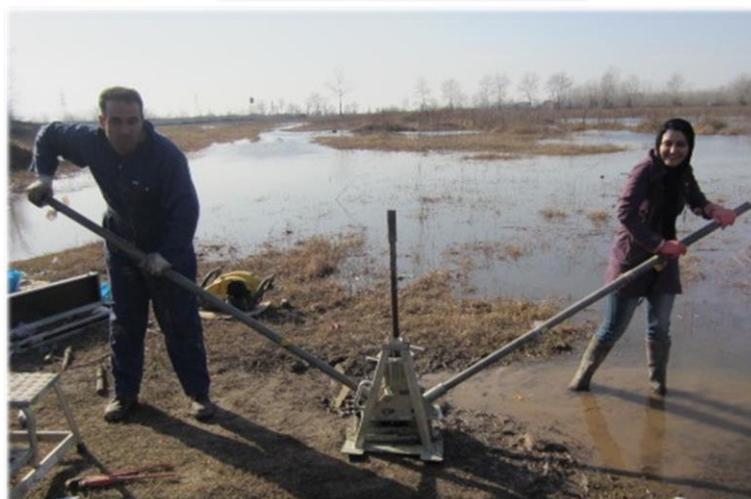
Fig. 3.4. Taking core from the land using the percussion corer (Photos: the Author). Left: going down. Right: extracting the core from the ground. Location: AAL13V, north of Astaneh Town.
