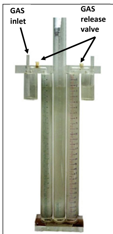
Figure 3.26: Fifth Gas measuring device.
