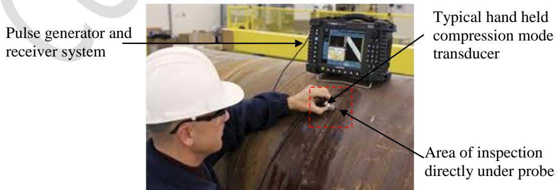
Figure 1-4. Conventional NDT inspection of weld integrity.
