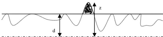
Figure B.6: Example of statistical model for contact between a rough surface and a smooth rigid plane.
