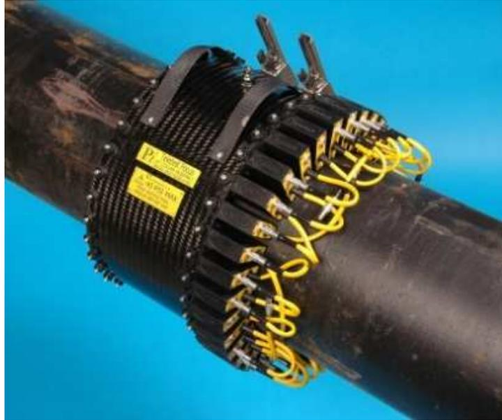
**Figure 1.2 Plant Integrity Guided Wave system for an 8” pipe.**
