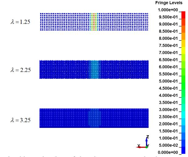
The increase in size of h resulted in reduction of the damage magnitude average and peak values
