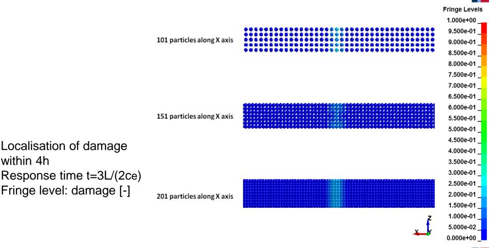
The damage effects propagated the same distance in all simulations, giving a constant softening zone size.
