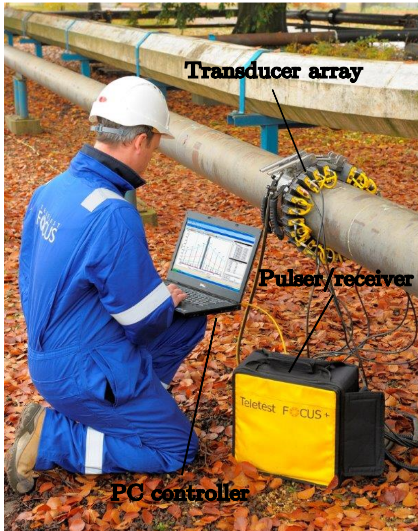
FIGURE 1.1: The Teletest Focus + GWT system showing the key components; the transducer array, the pulser/receiver and the PC controller.
