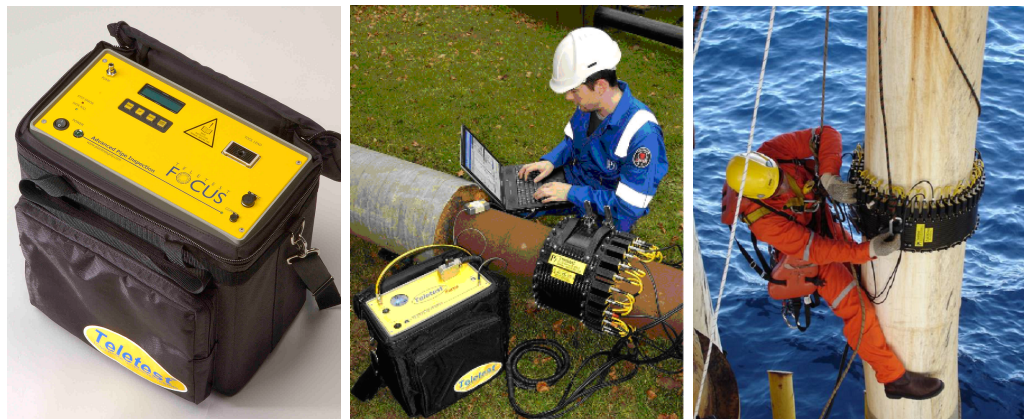
(a) Teletest ® MK3 Electronic Unit (b) Teletest ® MK3 System used in inspecting insulated pipeline (c) Teletest ® MK3 System used for testing off-shore riser
