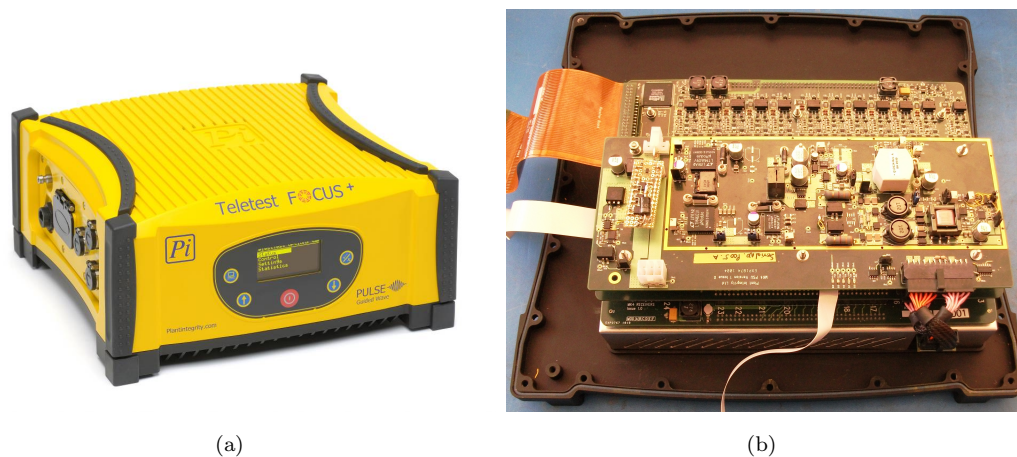
FIGURE 8.1: Teletest ® MK4 Electronic Unit and Internal Assembly of the First Prototype System
