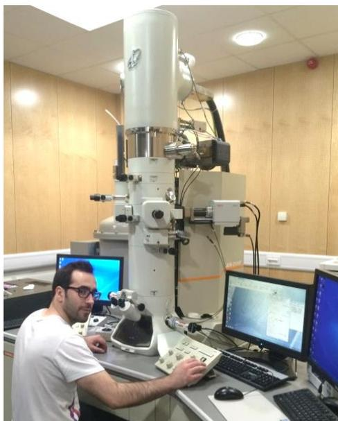
**Fig. 3.3** JEOL TEM-2100F (FEG-TEM) used in this study, located at the Experimental Techniques Centre (ETC), Brunel University London.
