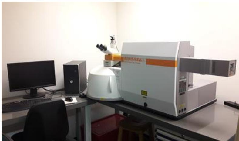
**Fig. 3.6** Renishaw's inVia confocal Raman microscope used in this study.
