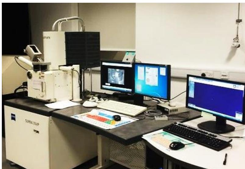
**Fig. 3.2** FEG-SEM Zeiss Supra 35VP used in this study.
