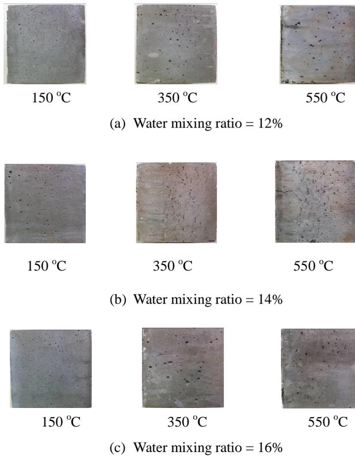
**Fig. 1** Surface appearance of the specimens after heating.
