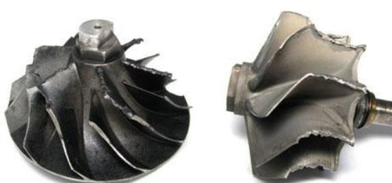
Figure 12: Foreign object damage [13].
