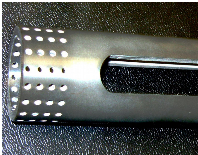
Figure 2.14. The ceramic rotor-stator impeller.
