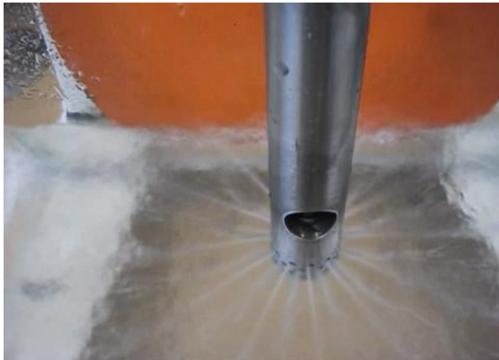
Figure 6.18. Jets around a new stator (crossH) are arranged uniformly in the space what improves the uniformity of a fluid agitation.
