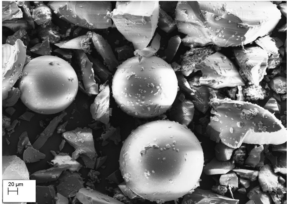
Figure 4.12. SEM picture of sheared alumina powder. We can observe some non-sheared particles of alumina and broken parts of spheres. As there are well defined so in cross-section of samples we observed sizes of single particles.
