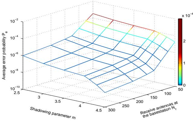
Fig. 4. The functional comparison among average bit error rate performance, channel parameter  $m$  and number of receive antennas for perfect CSI and differentially coherent DPSK detection ( $R_k = 600m$ ,  $P = 15dB$ ,  $\nu = 2.0$ ,  $a = 1$ ,  $b = 1$ ).
