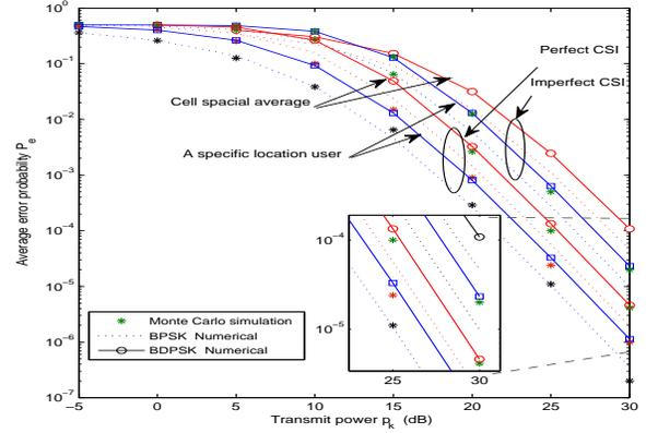
Fig. 1. Average bit error probability for single user located at  $R_k = 600m$  compared with spacial averaged user (entire cell) with Perfect/Imperfect CSI and different modulation ( $\nu = 3.3, m = 3.0, \tau = 4, N_r = 250$ ).
