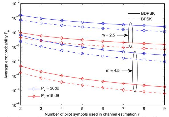
Fig. 2. Average bit error probability for single user located at  $R_k = 600m$  versus number of symbols used in training sequence of channel estimation ( $N_r = 150, \nu = 2.0$ ).
