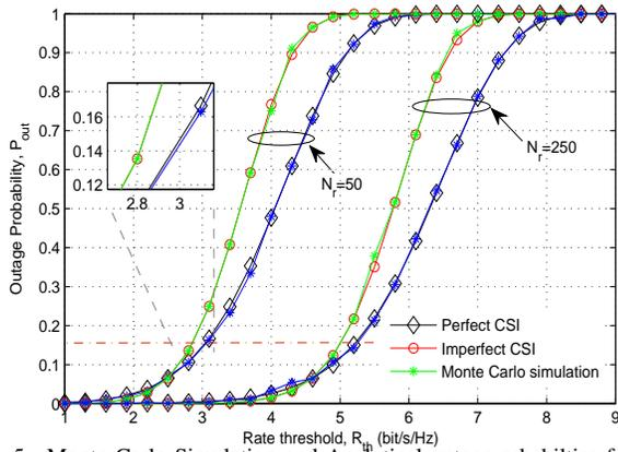
Fig. 5. Monte Carlo Simulation and Analytical outage probabilities for single user located at  $R_k = 600m$  from the base station with perfect/imperfect CSI and different number of base station antennas ( $P = 15dB$ ,  $\nu = 2.5$ ,  $m = 2.5$ ,  $\tau = 1$ ).
