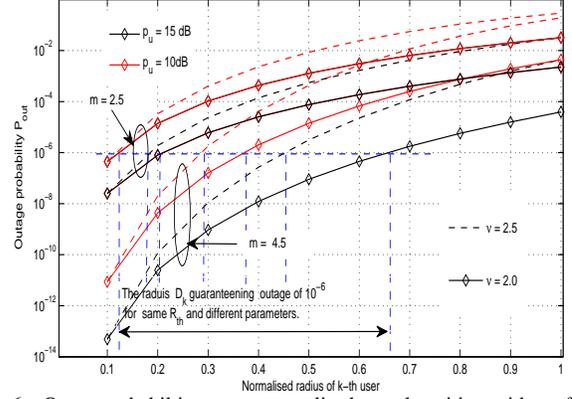
Fig. 6. Outage probabilities versus normalised user location with perfect CSI and different system parameters ( $N_r = 250$ ,  $R_{th} = 2.5b/s/Hz$ ).
