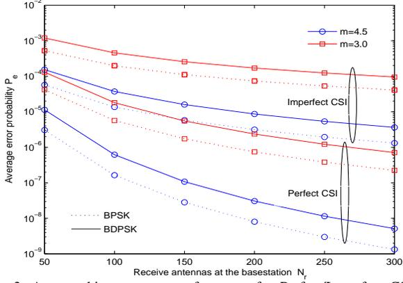
Fig. 3. Average bit error rate performance for Perfect/Imperfect CSI with different values of channel parameter  $m$  and two modulation schemes for single user located at  $R_k = 600m$  ( $P = 15dB$ ,  $N_r = 128$ ,  $\nu = 2.0$ ,  $m = 2.5$ ,  $\tau = 4$ ).
