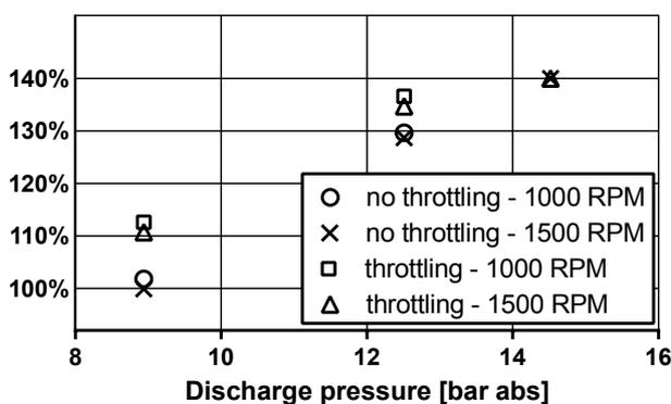
Figure 5: Oil flow rate at off design with respect to test # 7 of Table 3 (8.5 bar at 1500 RPM)
