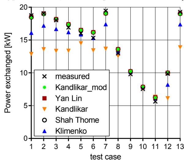
Figure 3: Model validation on thermal power exchanged
