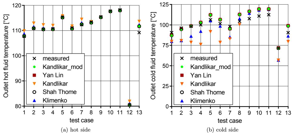
Figure 2: Comparison between measured outlet temperatures with model results obtained using different correlations for the phase change of the organic fluid
