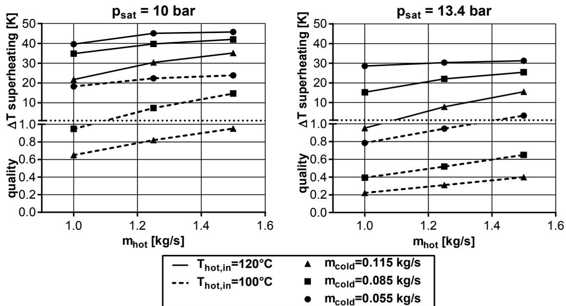
Figure 6: Effects of off-design operating conditions of a plate heat exchanger for waste heat recovery in terms of quality and superheating or subcooling of the organic fluid at the heat exchanger outlet
