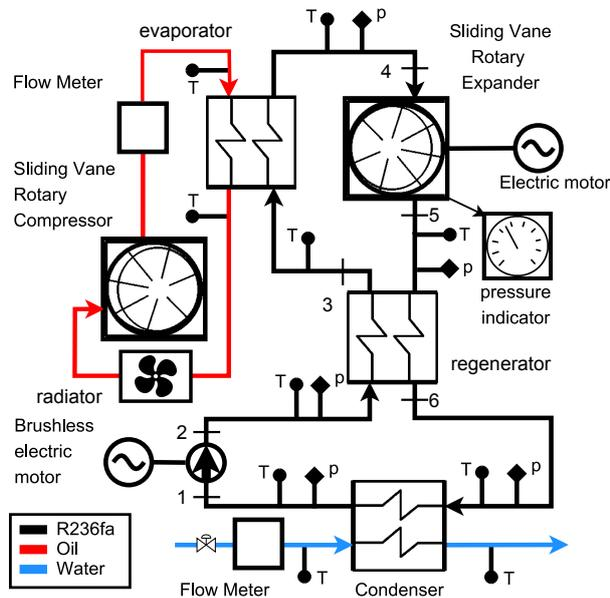
Figure 1: ORC system test bench with sensors layout
