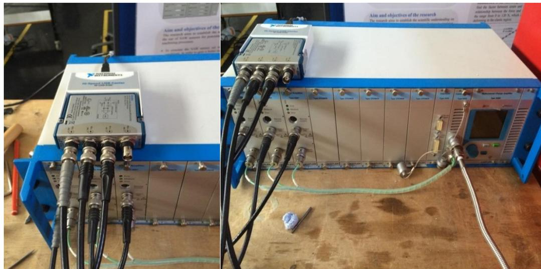
Figure 4-8: The data collection and multichannel charge amplifier
