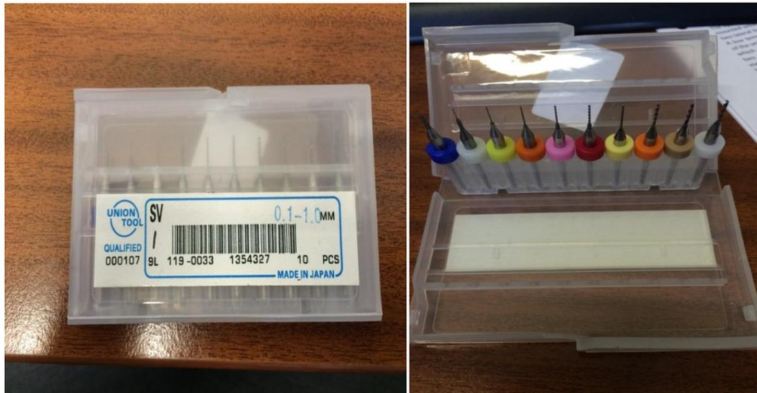
Figure 4-15: PCB Tungsten carbide drill tool
