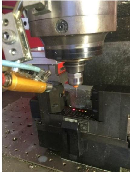
Figure 4-23: Laser tool position measuring system
