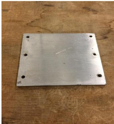
Figure 4-17: Al/Cu metal matrix composite
