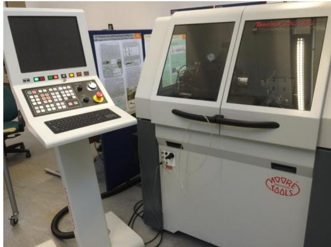
Figure 4-20: NANOTECH 250UPL Ultra-precision Lathe
