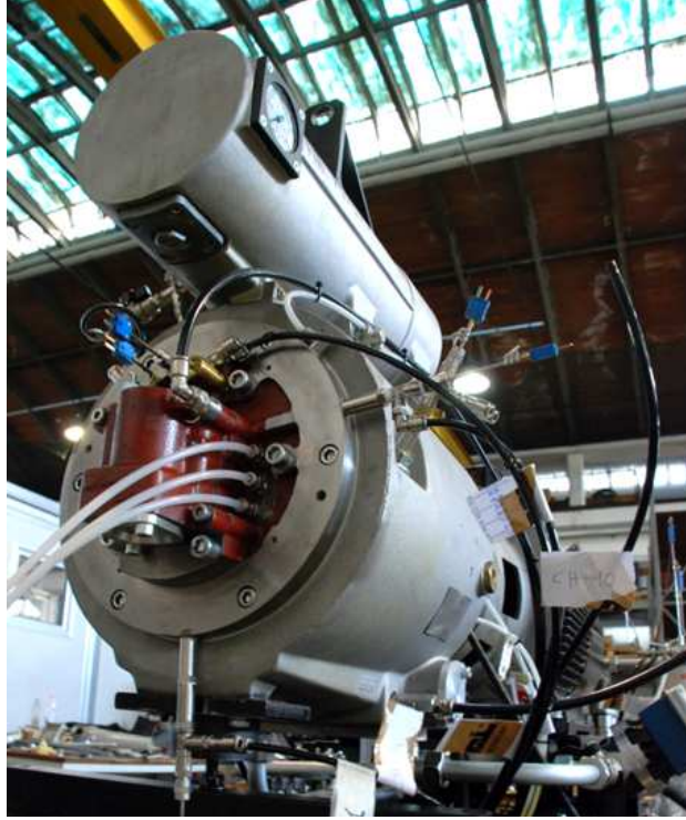
Figure 5: Mid-size sliding vane compressor equipped with three pressure-swirl injectors installed on an endwall plate and fed through the white colored high pressure pipes (the remaining two atomizers were installed on the opposite side cover)
