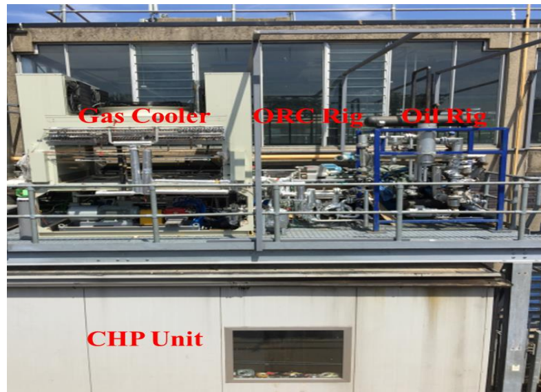
Figure 3.5 R245fa ORC test rig with heat source system in Brunel University London.
