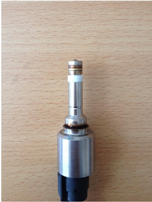
Figure 3-7: Multi-hole solenoid injector external (left) and internal (right) views
