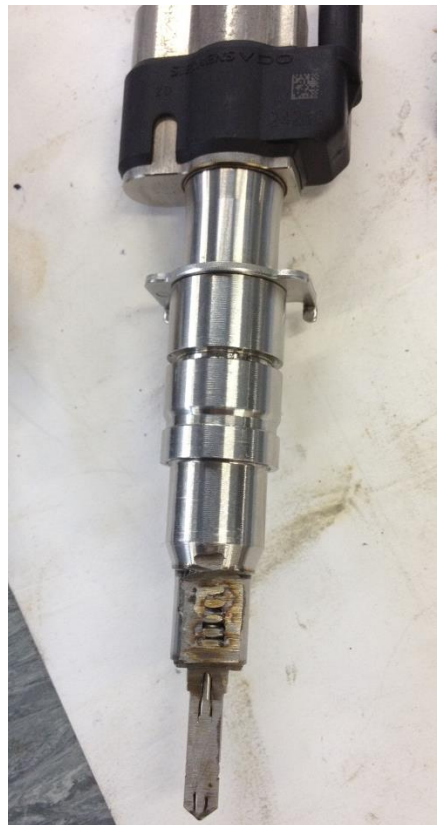
Figure 3-8: Piezo type injector external (left) and internal (right) views
