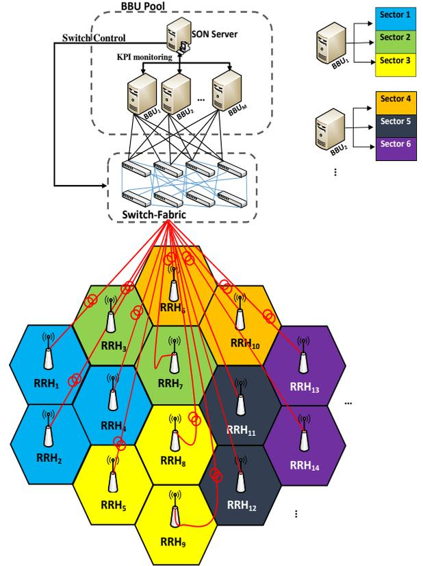
Fig. 2. Structure of a Cloud Radio Access Network represented as SON
