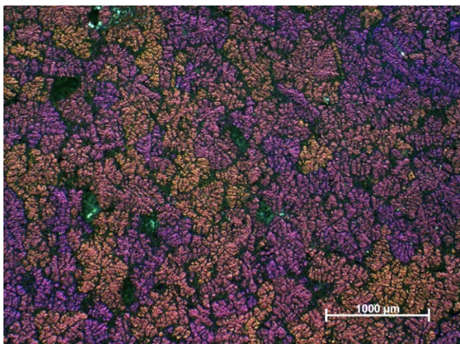
Figure A - 42 Anodised microstructure of A356, with 1.0% wt. Al-2Nb-B addition, taken at 30mm from the tip of the wedge mould, showing grain size.
