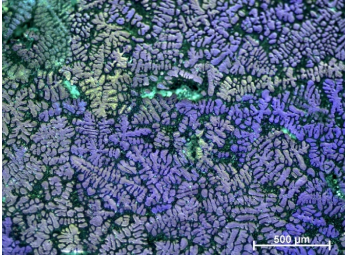
Figure A - 20 Anodised microstructure of A356, with 0.1% wt. Al-2Nb-B addition, taken at 10mm from the tip of the wedge mould, showing grain size.
