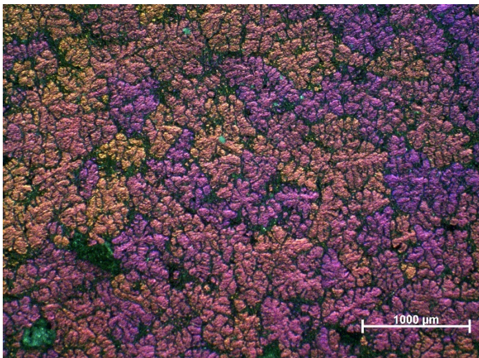
Figure A - 47 Anodised microstructure of A356, with 1.0% wt. Al-2Nb-B addition, taken at 80mm from the tip of the wedge mould, showing grain size.
