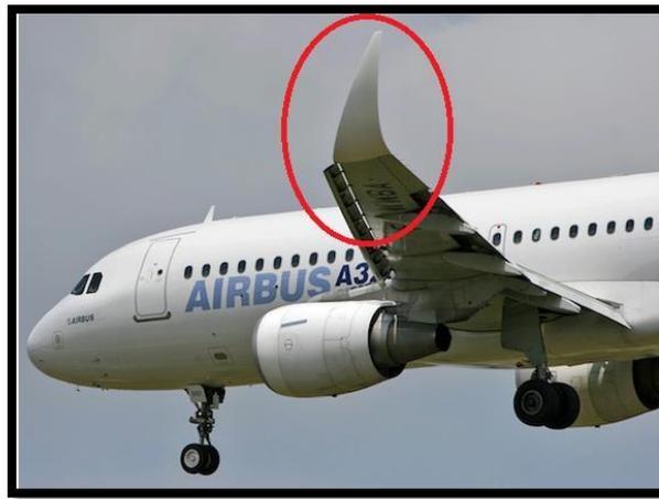
**Figure 2.43** Installed Sharklets on Airbus A-320 family [108].
