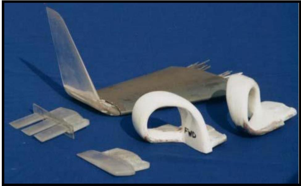
**Figure 2.38** The wing model including winglet shapes [95].
