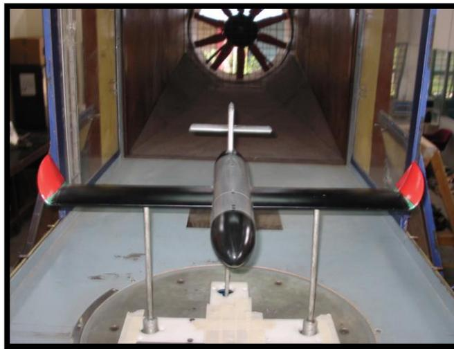
**Figure 2.39** Hossain[100] elliptical winglet configuration with  $60^\circ$  cant angle.
