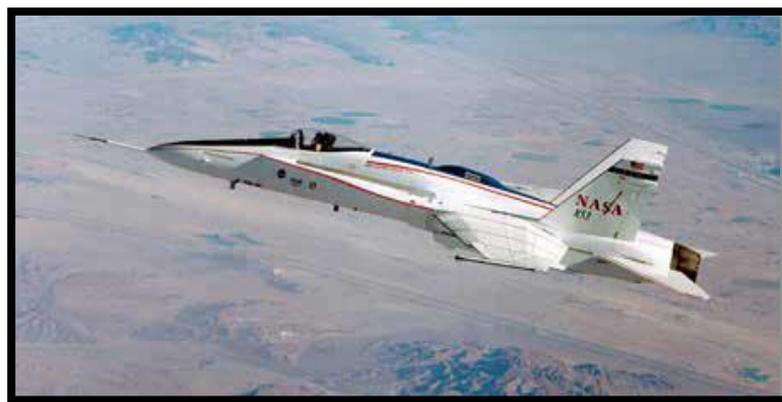
**Figure 2.13** NASA Dryden Flight Research Center F/A-18 with flexible wing [21].
