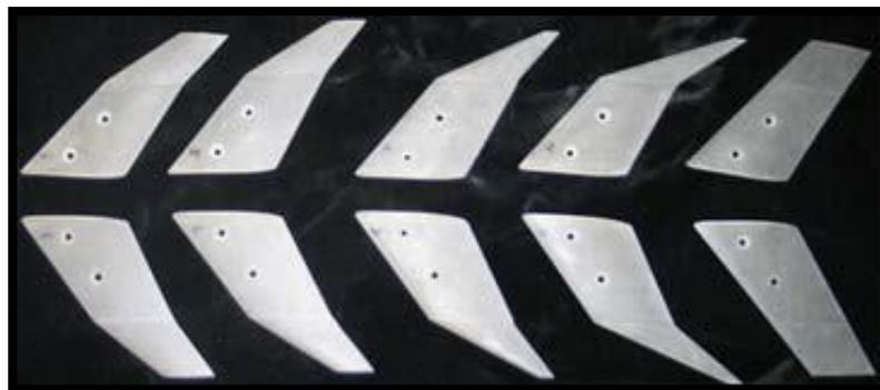
**Figure 2.40** Various raked wingtip test models : Raked angle of  $15^\circ$ ,  $20^\circ$ ,  $25^\circ$ ,  $30^\circ$ , and  $0^\circ$  from Left to right [102].
