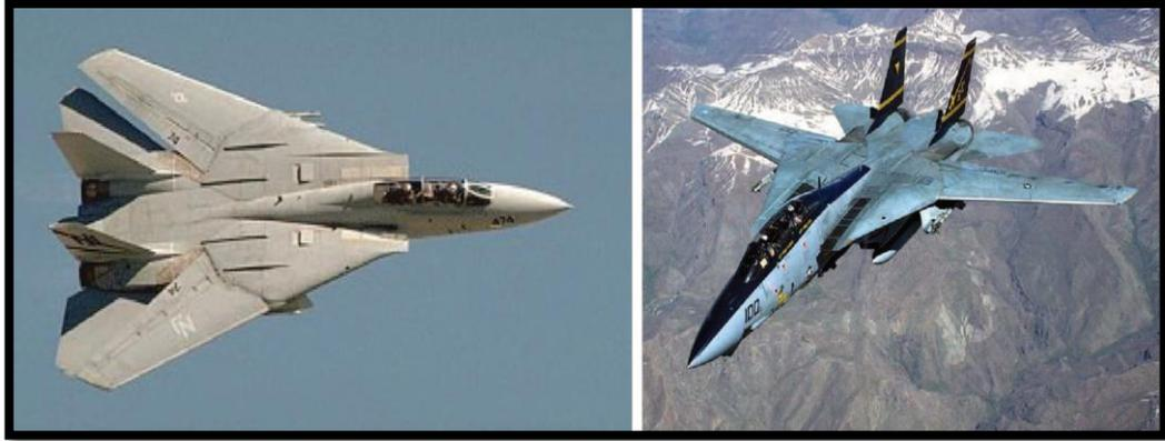
**Figure 2.10** F-14 Tomcat: sweep back position (Left) and un-swept configuration (Right) [19].
