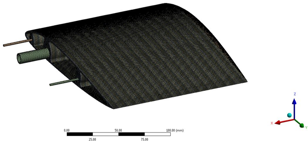
**Figure 3.16** Applied appropriate meshing size to morphing elements.
