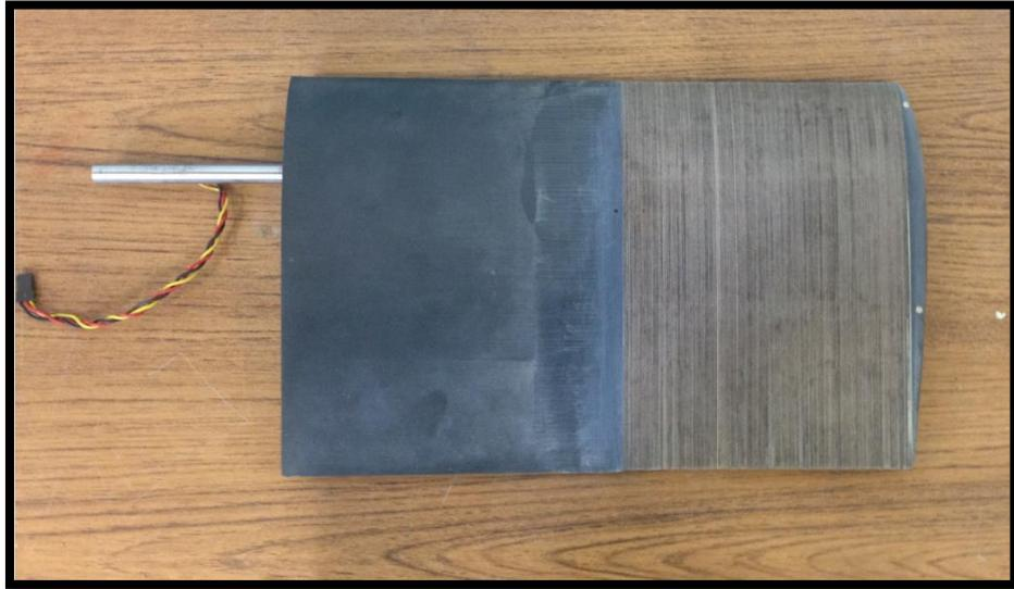
**Figure A- 3** Sanded Wing and Morphing Structure.
