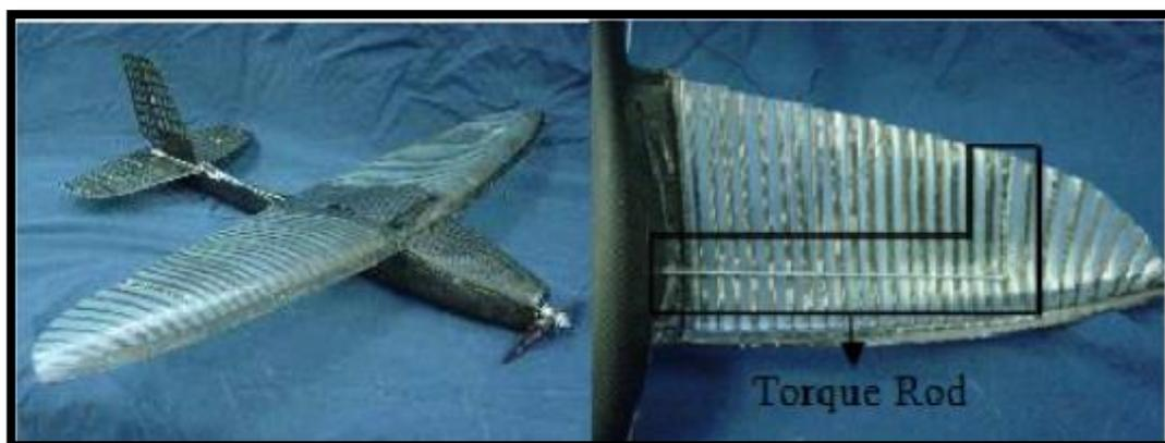
**Figure 2.31** Review of Garcia[68] design: micro air vehicle (left) and (b) torque rod assembled membrane wing (right).
