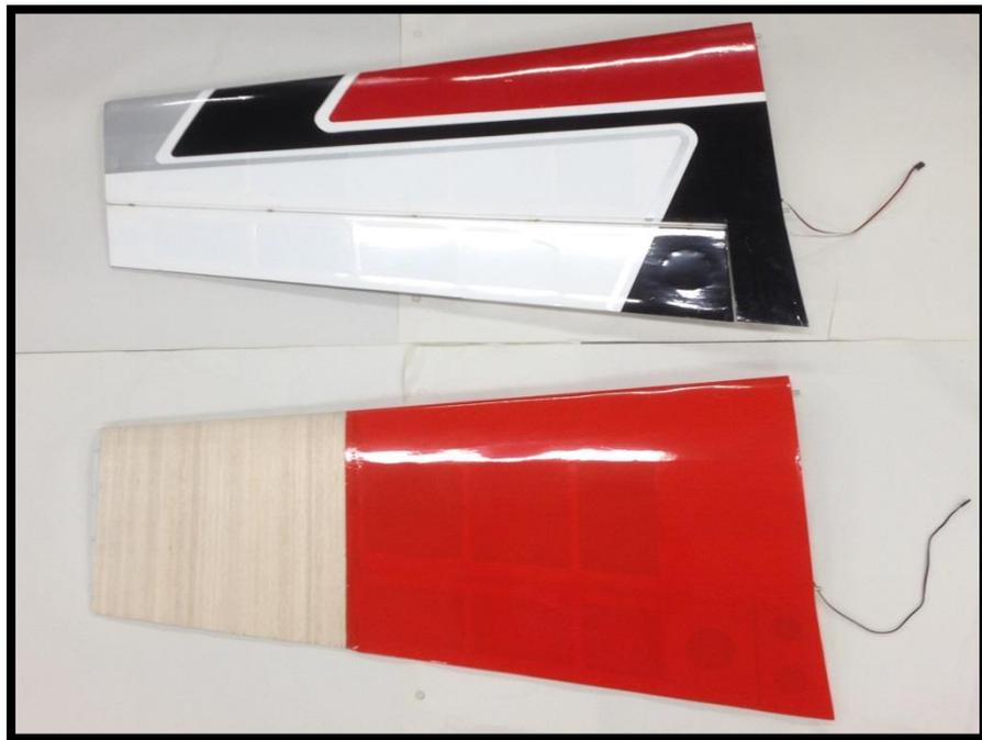
**Figure 4.48** Wing Structures: Fixed wing with an aileron (top side) and wing with twist section (bottom side).
