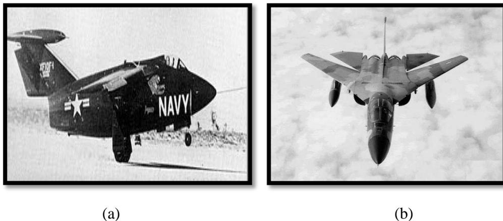
**Figure 2.9** Variable sweep wing aircraft: (a) XF10F-1 Jaguar (1952) [17] and (b) F-111 Aardvark (1964) [18].
