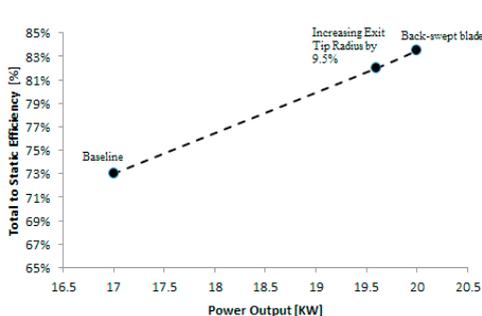
Fig. 4a: Efficiency Improvement of the radial turbine
