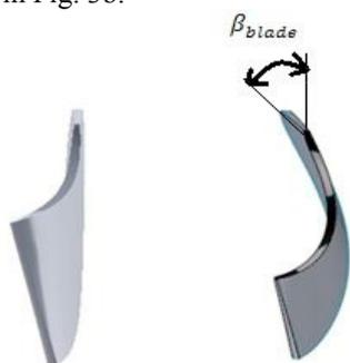
Fig. 3a: (left) radial blade (right) non-radial blade
