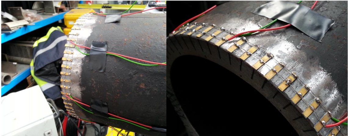
Figure 5.22. High density transducer array with 64 piezoelectric elements.
