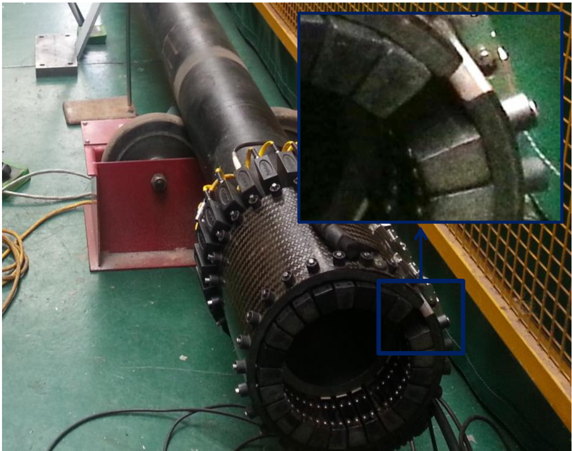
Figure 5.4. Existing transducer array coupled to a 6 inch schedule 120 pipe showing the gap in the transducer array.
