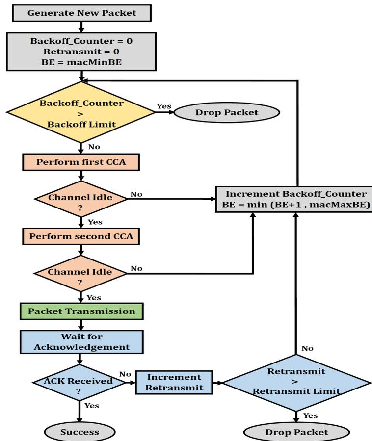
Figure 3.1: Block diagram of an unslotted CSMA/CA for 6LoWPAN [143]
