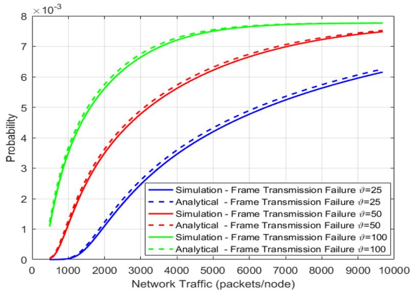
Figure 3.8: Frame transmission failure probability versus network traffic
