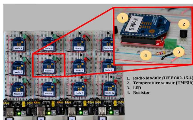
Figure 5.1: Simple node prototype
