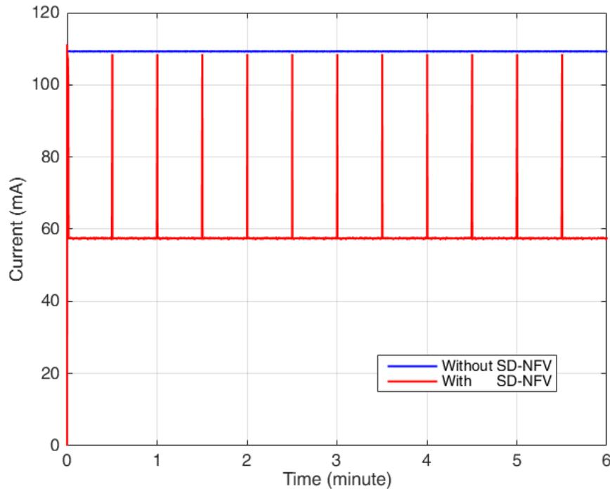
Figure 5.15: Current drawn from 6LoWPAN node under a periodic traffic condition
