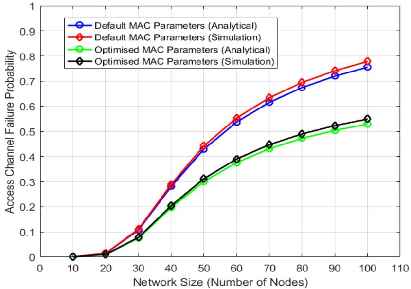
Figure 3.24: Access channel failure probability
