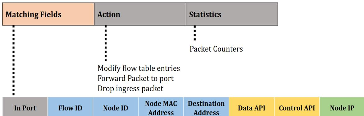
Figure 5.8: The proposed flow table entries of the customised SDN controller
