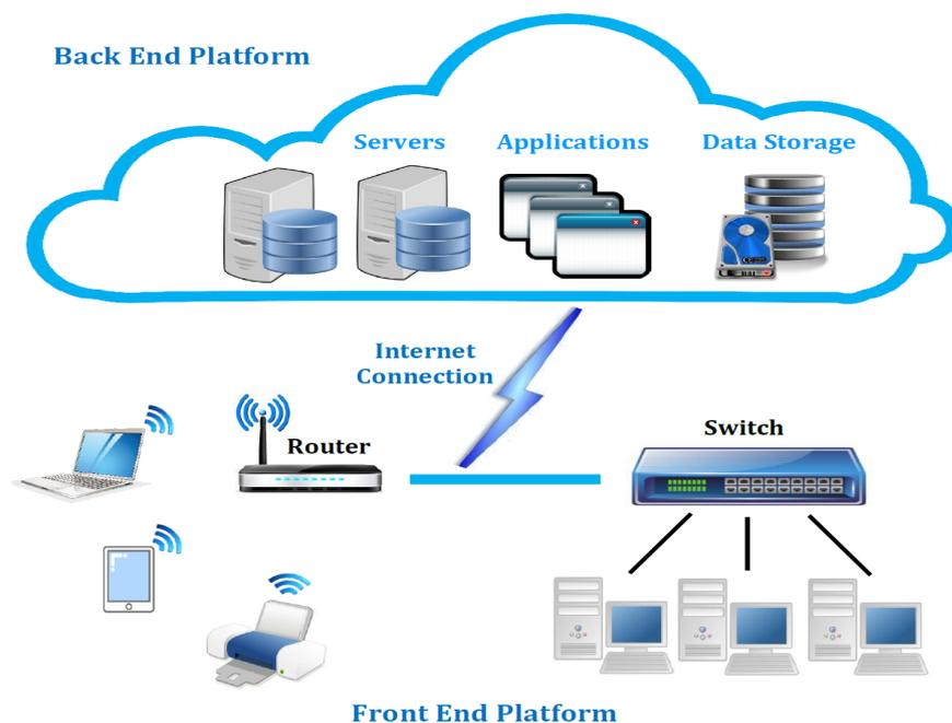
Figure 2.9: Cloud computing architecture
