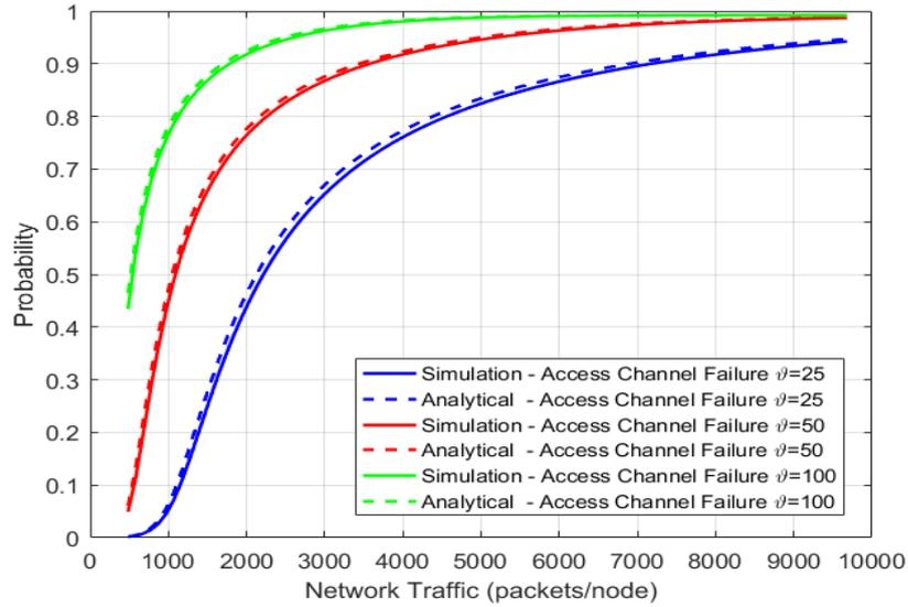
Figure 3.7: Access channel failure probability versus network traffic
