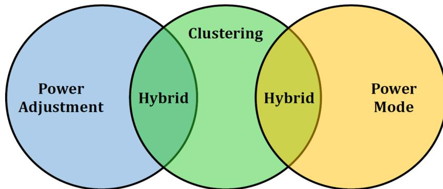
Figure 2.4: The four categories of topology control techniques in sensor networks
