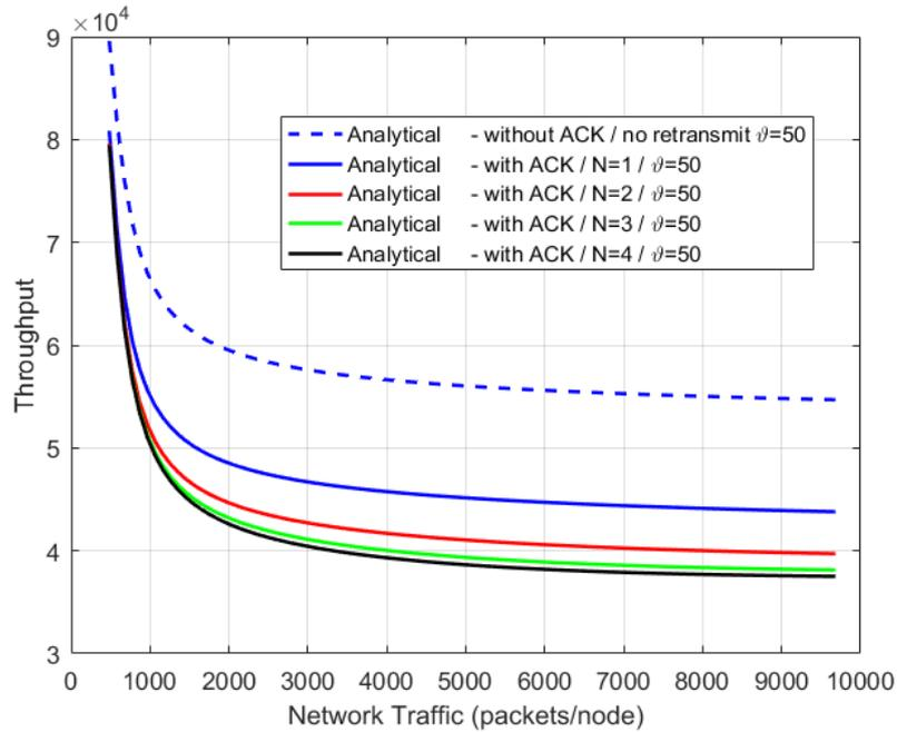
Figure 3.9: Instantaneous throughput with retransmission versus network traffic
