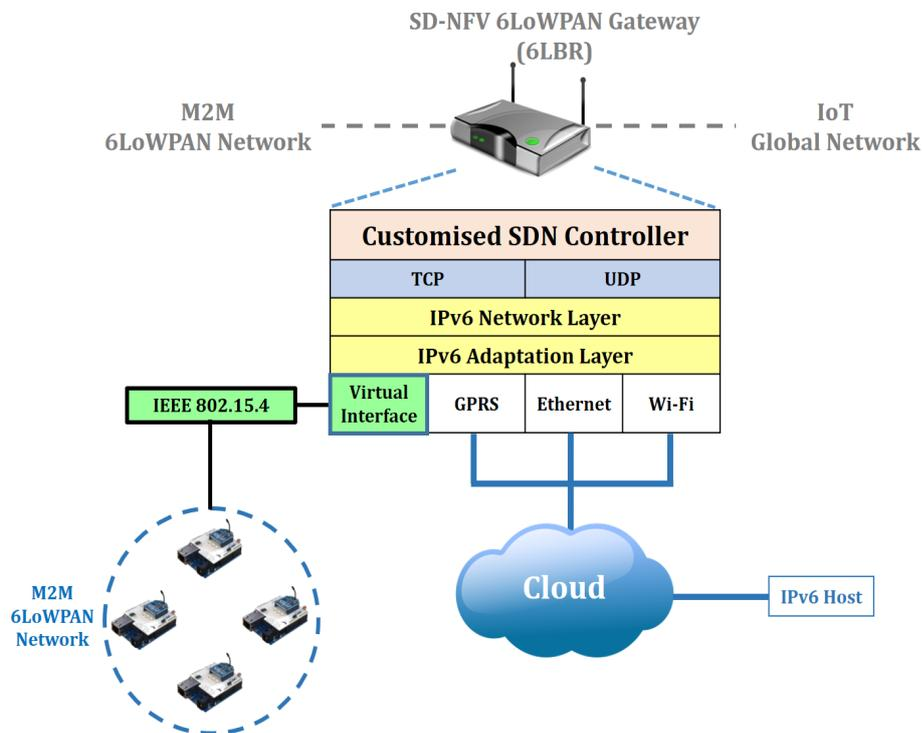
Figure 5.10: 6LoWPAN cloud connectivity through the SD-NFV gateway
