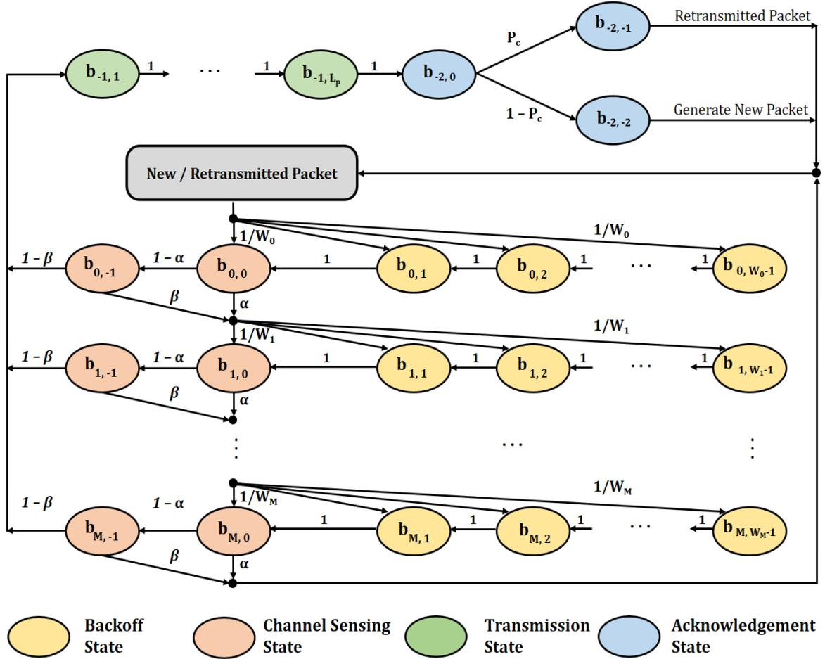
Figure 3.2: Markov chain model for CSMA/CA of IEEE 802.15.4 standard per single transmission attempt [148]
