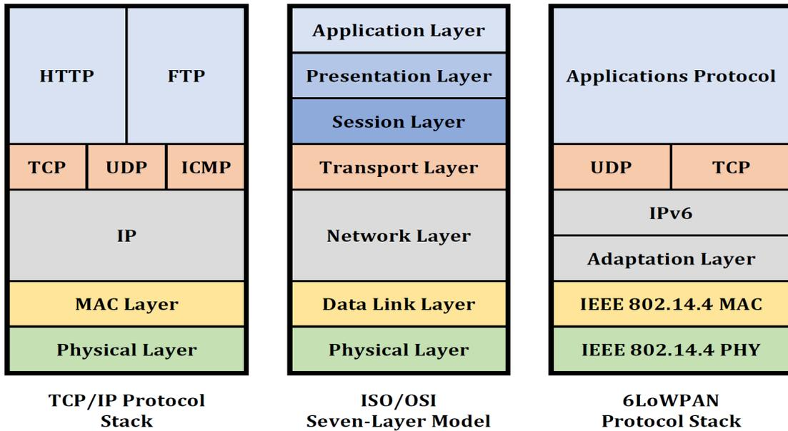
Figure 2.3: Protocol stack of TCP/IP, OSI model and 6LoWPAN [16]
