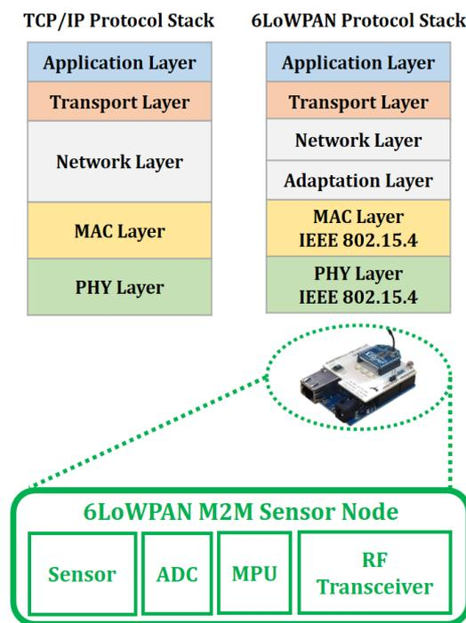
Figure 5.4: M2M sensor node architecture
