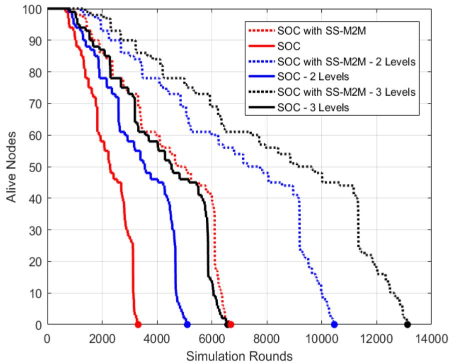
Figure 4.12: M2M sensor network lifetime with smart sleep scheduling
