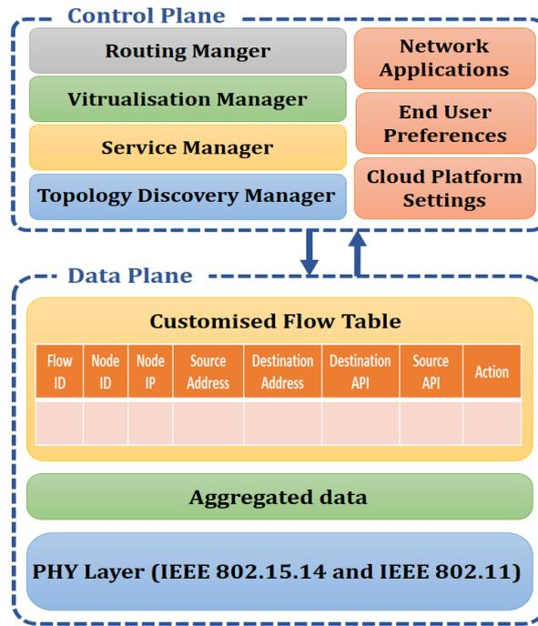
Figure 5.5: Customised SDN controller architecture
