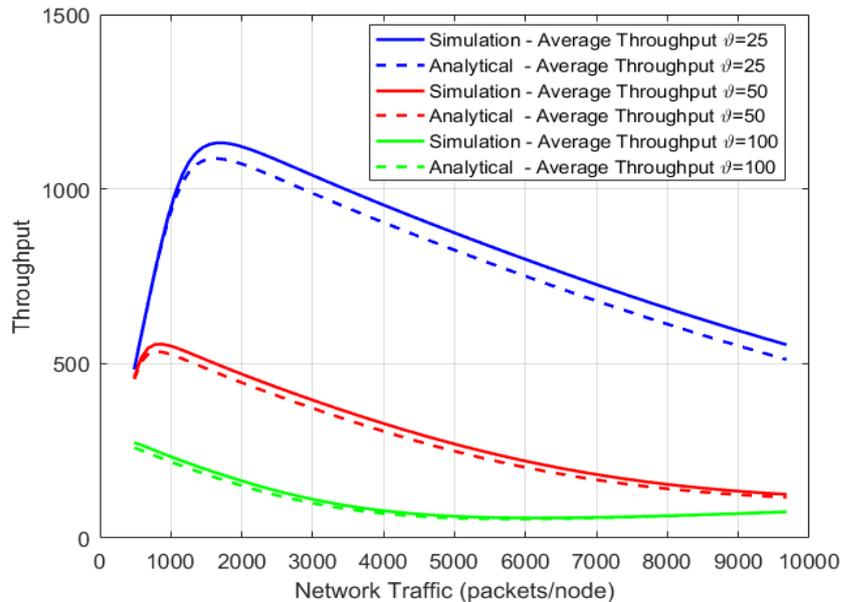
Figure 3.6: Average throughput versus network traffic
