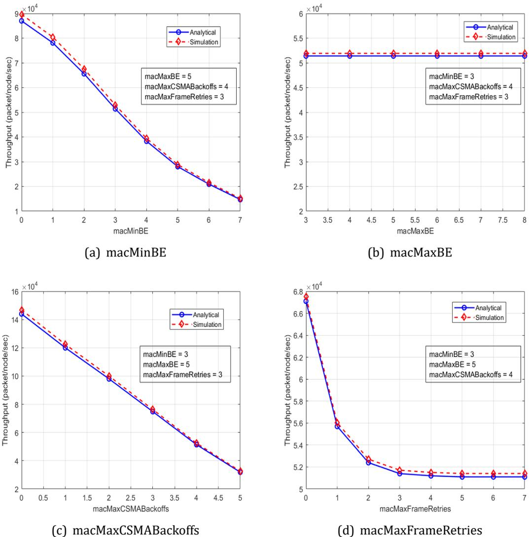
Figure 3.20: The effect of the MAC layer parameters for 50 node network size and offered load of 1,000 packet/node
