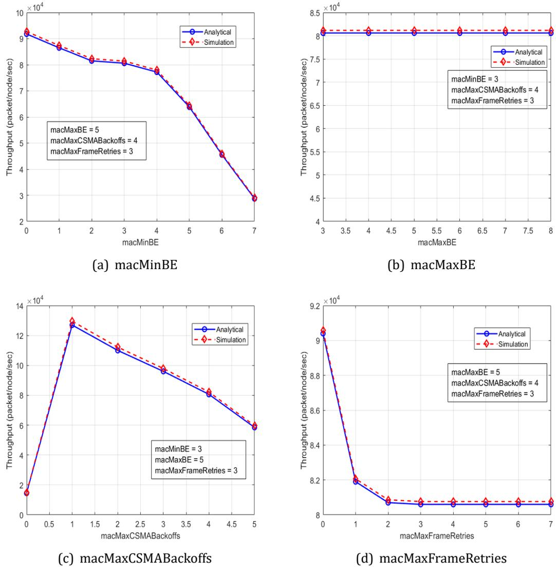
Figure 3.21: The effect of the MAC layer parameters for 100 node network size and offered load of 1,000 packet/node
