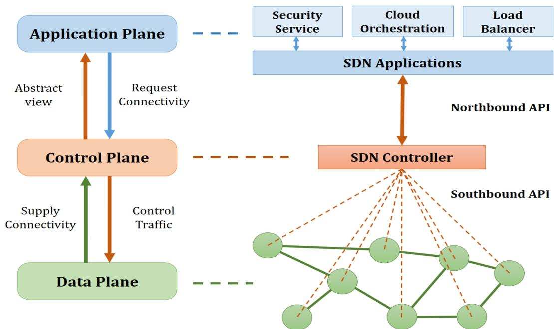
Figure 2.7: High-level SDN architecture
