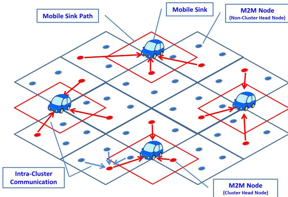
Figure 4.3: M2M sensor network architecture
