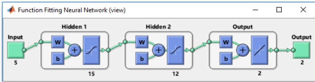
Figure 3.16: The best ANN topology obtained from the input/output pairs
