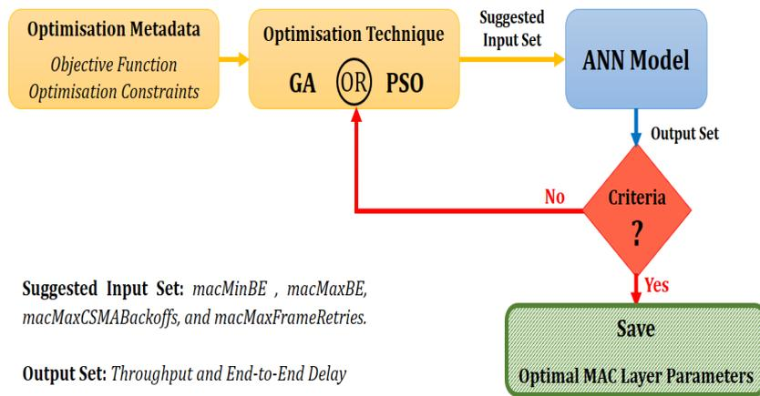
Figure 3.15: ANN-based optimiser for MAC layer parameter selection
