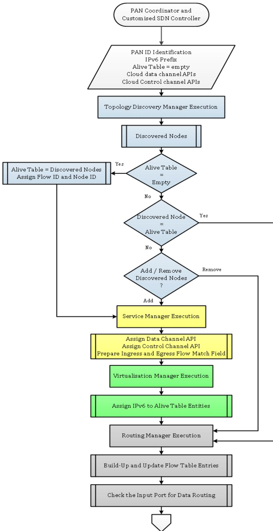
Figure 5.6: Implementation process of the customised SDN flow table
