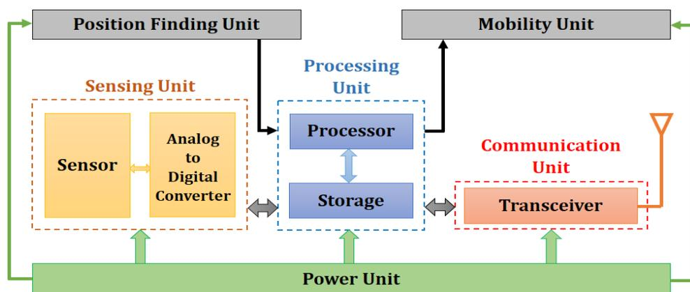
Figure 4.1: M2M sensor node architecture
