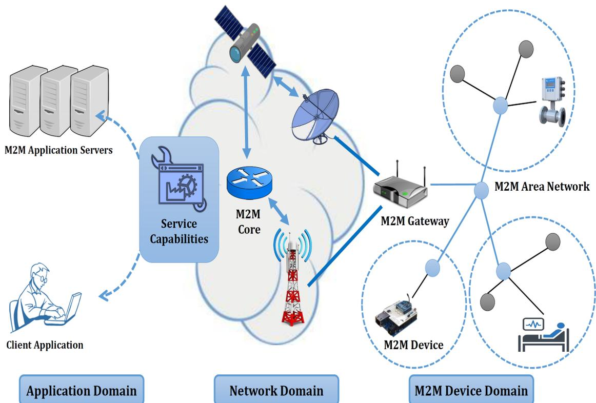
Figure 1.1: M2M communication architecture [11]
