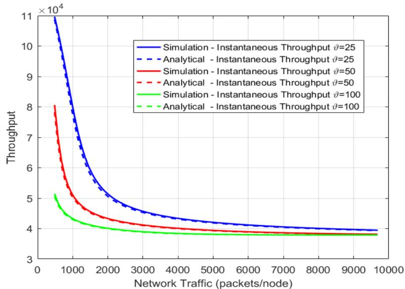
Figure 3.5: Instantaneous throughput versus network traffic
