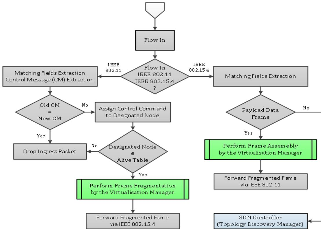
Figure 5.7: Implementation process of the customised SDN flow table (continued)
