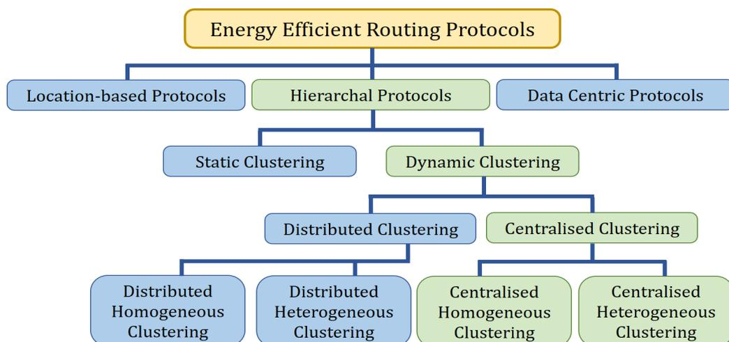
Figure 2.5: Classification of energy efficient routing protocols
