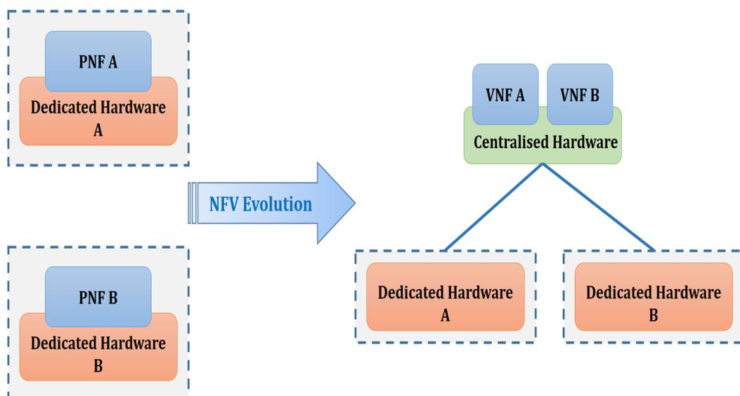
Figure 2.8: Basic NFV architecture
