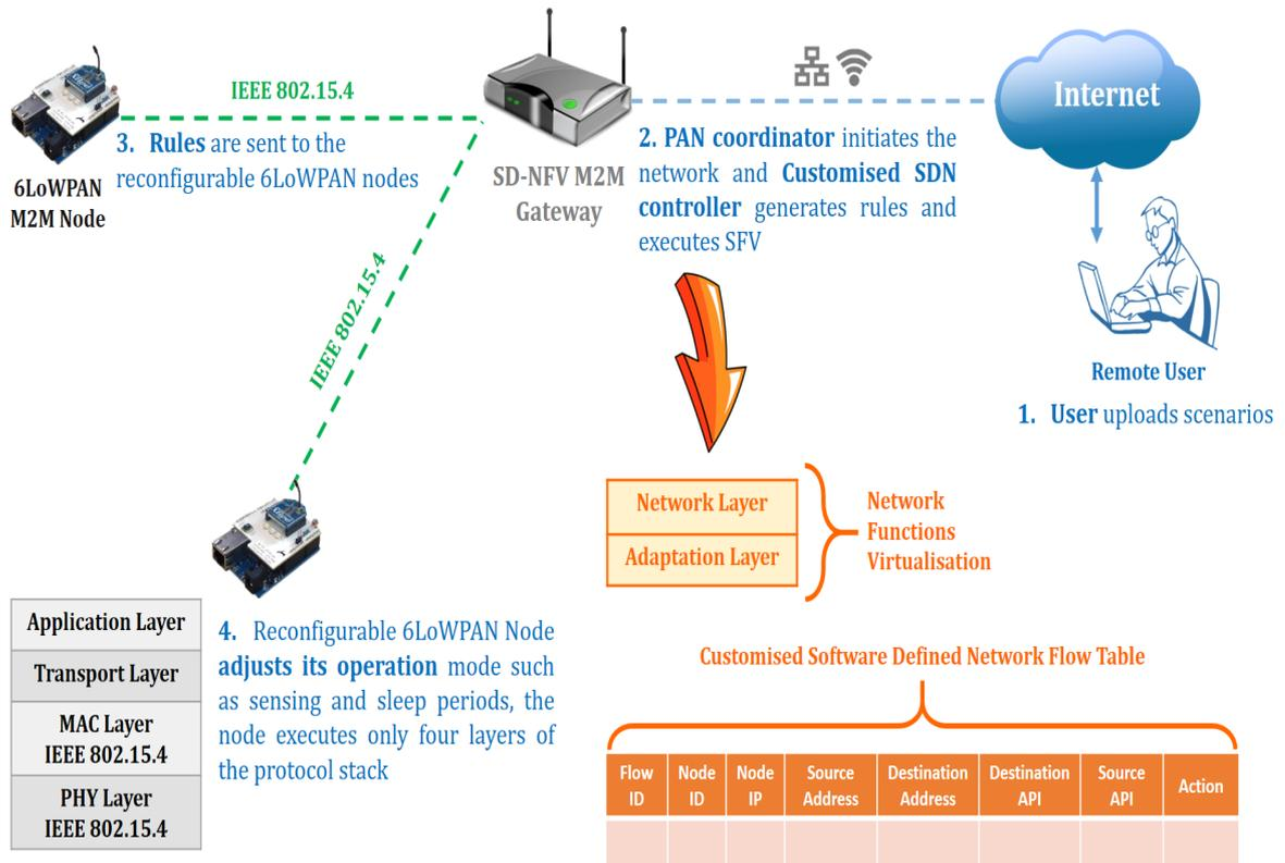
Figure 5.9: The proposed SD-NFV architecture based-on a 6LoWPAN testbed
