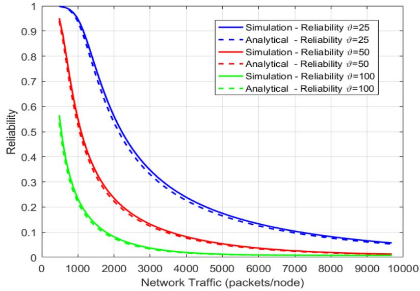
Figure 3.4: Reliability versus load offered
