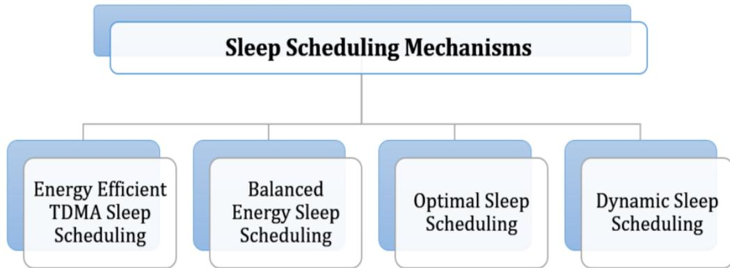
Figure 2.6: Classification of sleep scheduling mechanisms
