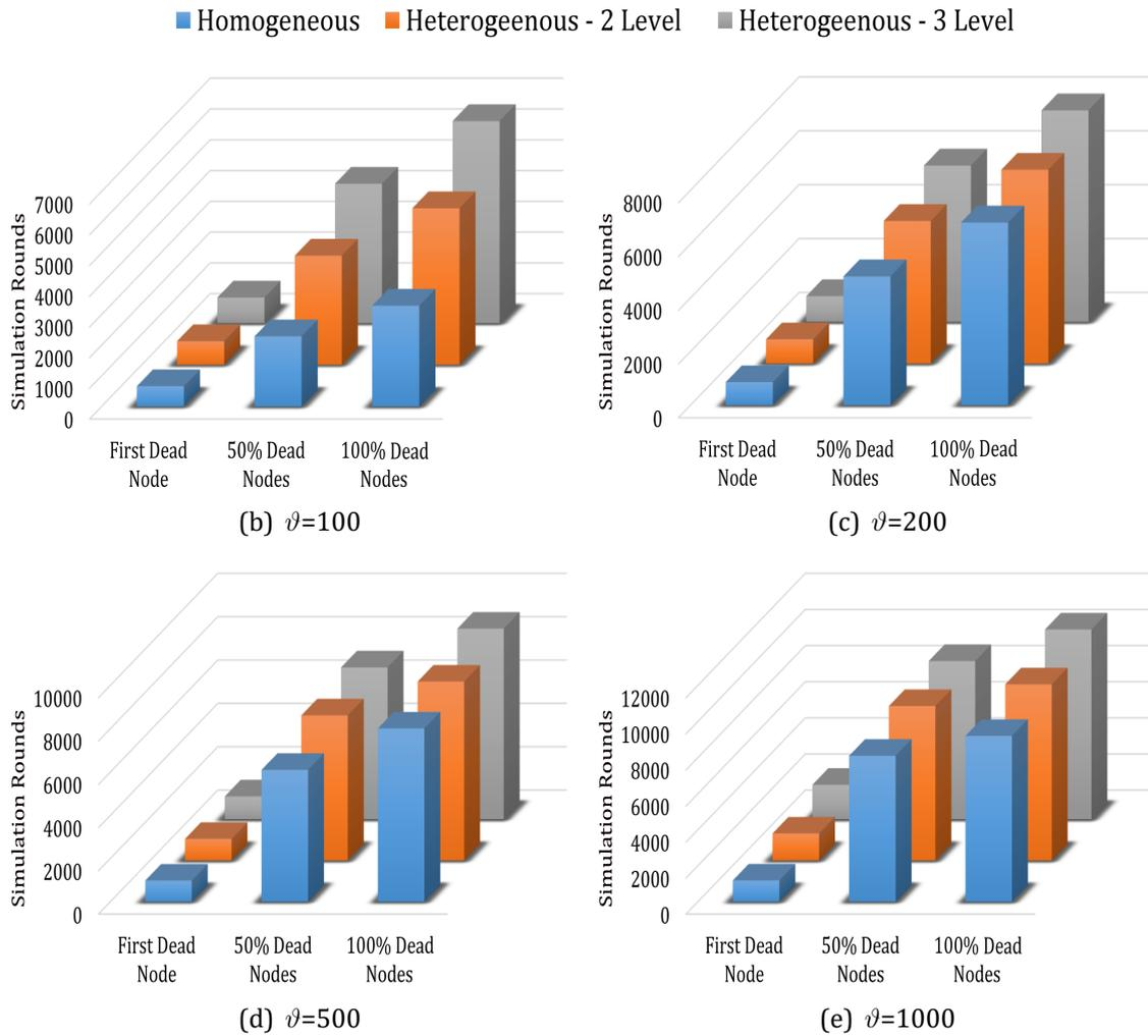
Figure 4.9: The scalability of the proposed energy-efficient SOC protocol
