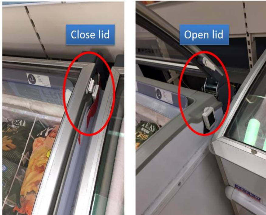
Figure 3-19: Hobo state data logger installed on the lift up lid frozen food cabinet
