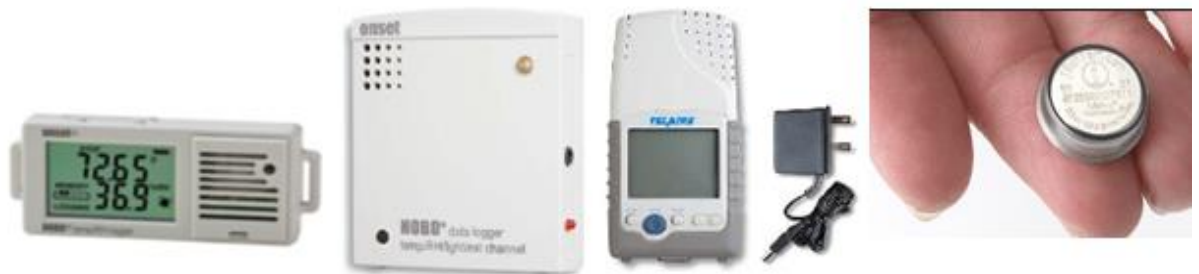
Figure 3-5: Monitoring equipment used for air temperature, relative humidity and CO 2 levels
