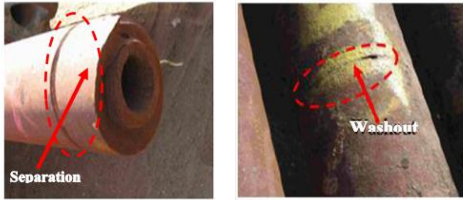
Figure 2.3: Drill string separation and drill string washout (Fesmi Abdul Majeed 2013)
