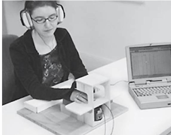
**Figure 3.10** Presentation of vibrations through the vibrator embedded in a small frame house (Source: Pongrac, 2008)
