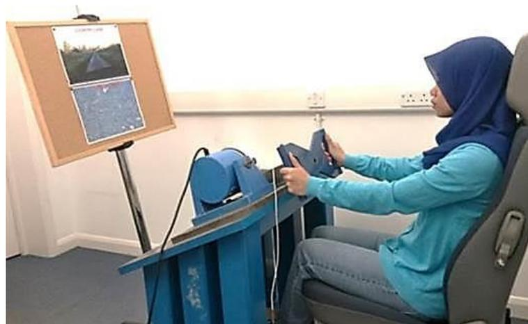
**Figure 7.2** Posture of participant at the steering wheel simulator
