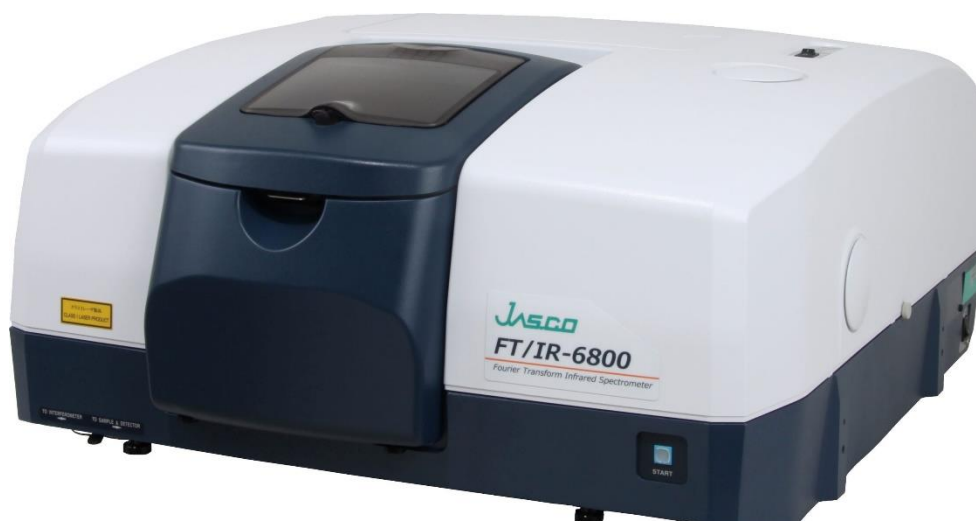
Figure 4. A photo of FTIR analytical tool used for bio-oil analysis.
