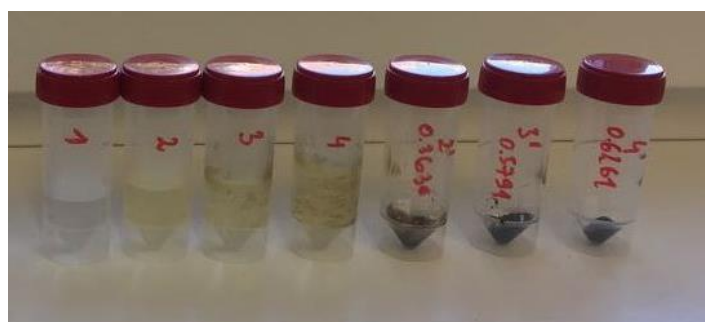
Figure 3. Pyrolysis liquid and oily samples taken from the pyrolysis reactor.
