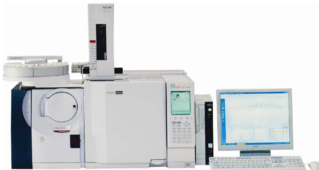
Fig. 5. Photo of GC/MS analytical tool used for bio-oil analysis.
