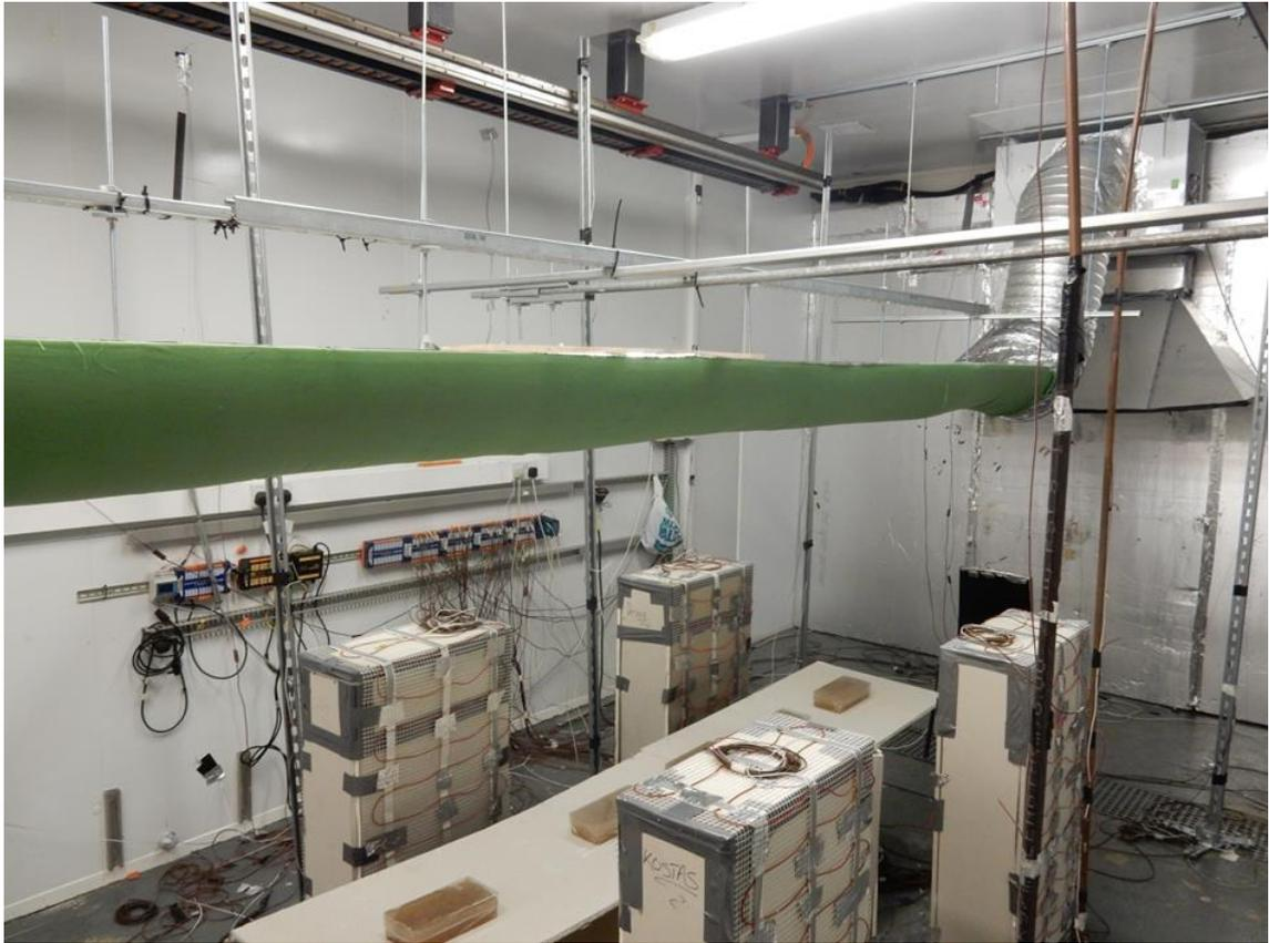
*Figure 7-1. Semi-circular fabric duct at medium level*
