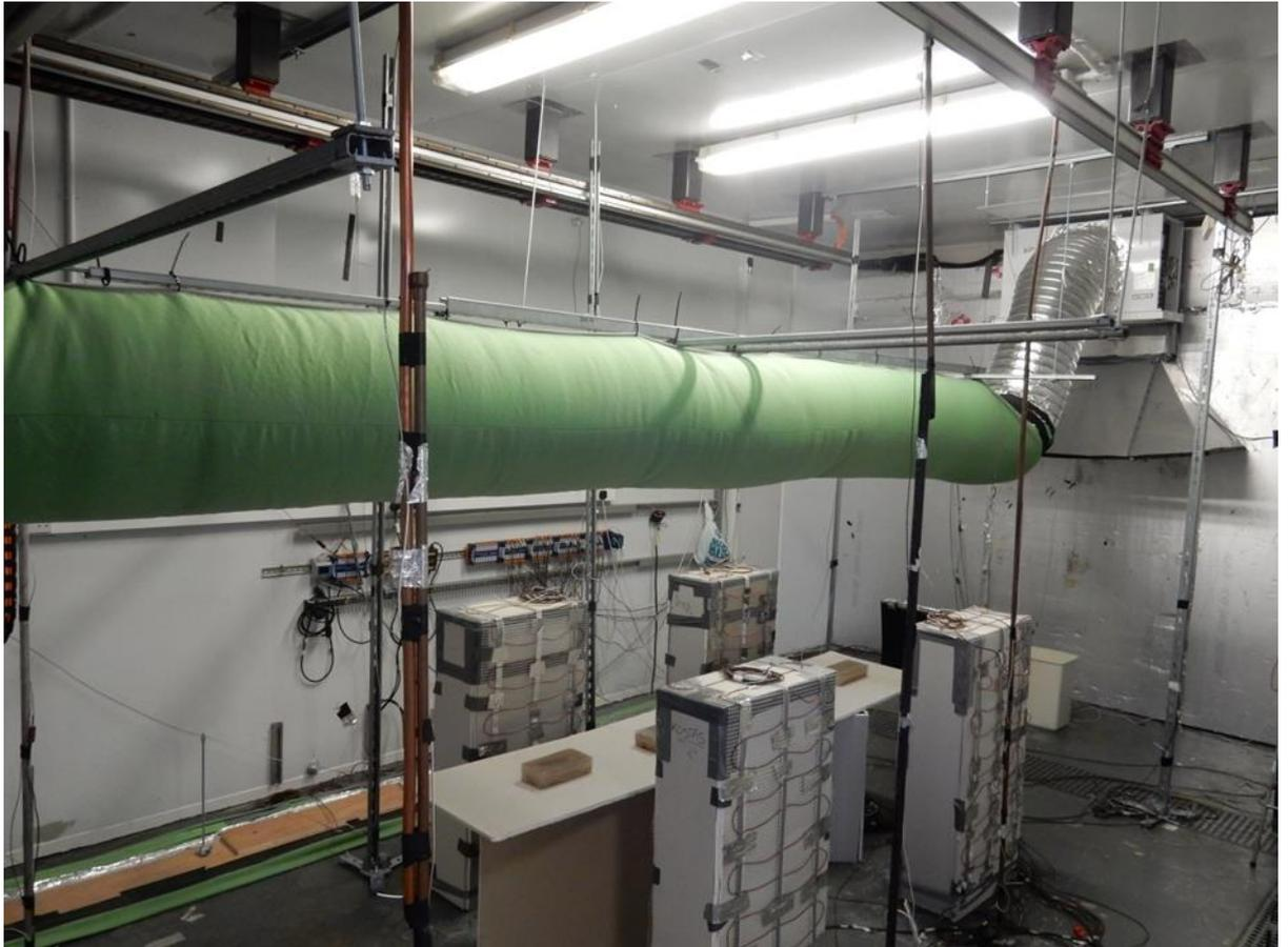
*Figure 7-14. Circular fabric duct at medium level*
