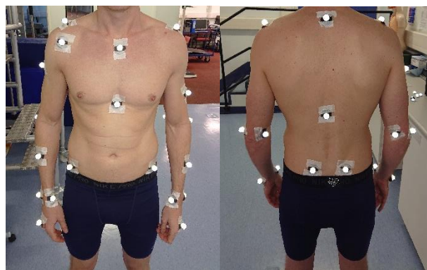
Figure 4-1: Marker set on the upper body, anterior view (left) and posterior view (right).
