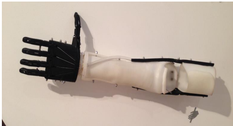
Figure 30: Project Daniel for upper limb prosthesis
